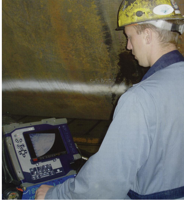
Figure 5 - From Insight, photo of phased array weld inspection using S-scan.
