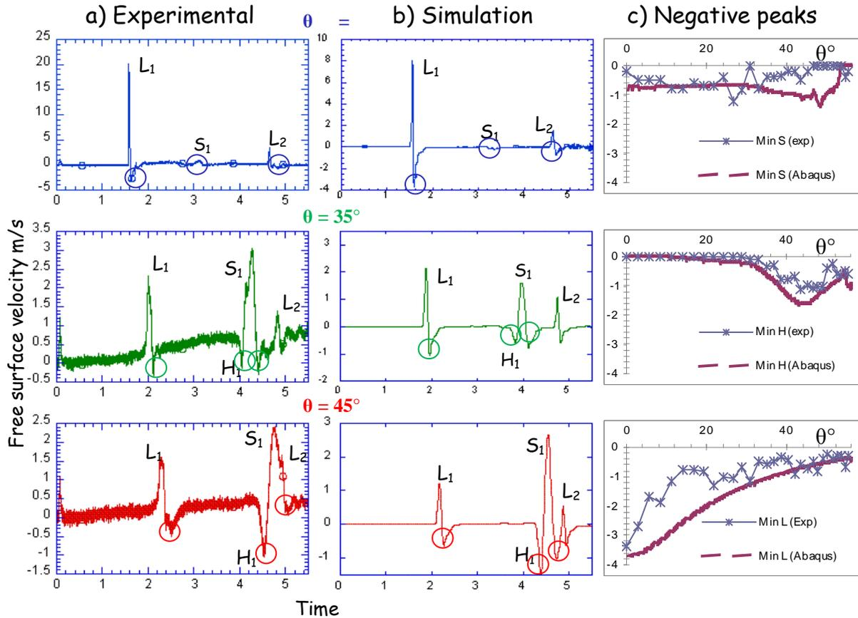
Figure 4. Free surface velocities corresponding to B-scan cuts: a) experiments, and b) simulations. c) Evolution of negative peaks for each wave (S1, H1 and L1 from top to bottom) at an angle  $\theta$ .
