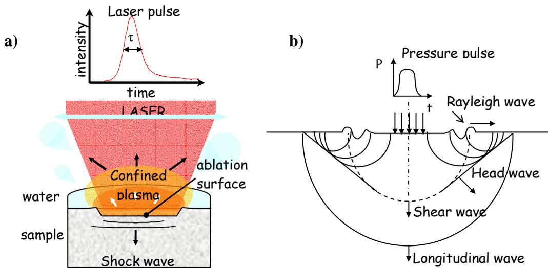
Figure 1. a) Laser-matter interaction in confined regime and b) different type of waves in metals.
