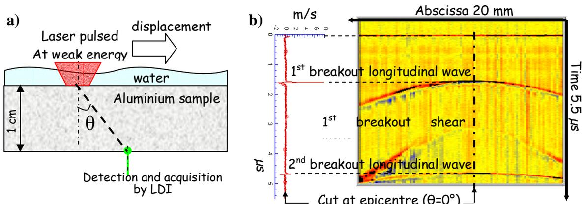
Figure 2. a) Experimental setup and b) B-scan with the velocity signal at epicentre.
