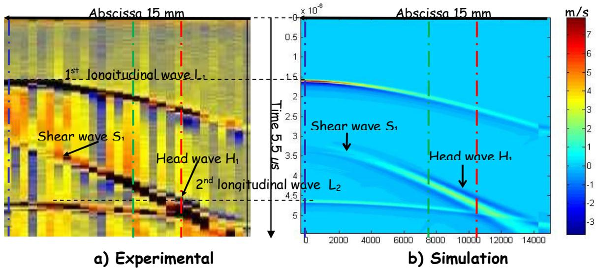
Figure 3. a) Experimental B-scan on an Al sample 1 cm thick and b) B-scan obtained with Abaqus. Vertical dashed lines are locations of velocity signals in Figure 4.
