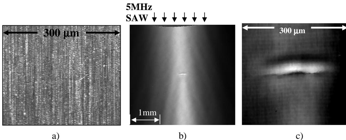
Figure 3. a) Digital image of titanium surface with surface-breaking crack at 100x magnification, b) displacement-field image of crack, and c) detailed DFI scan image of crack region.
