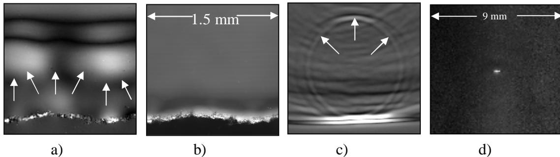
Figure 4. Displacement-field images based on: far-field scattering effects a) and c); and near-field scattering effects b) and d), for two different crack types.
