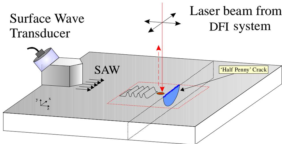
Figure 1. Schematic diagram depicting measurement process for Displacement-Field Imaging method.
