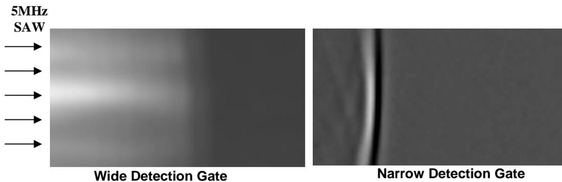
Figure 2. Examples of time-averaged (Left) and instantaneous (Right) displacement-field images taken with wide-gate and narrow-gate detection, respectively.
