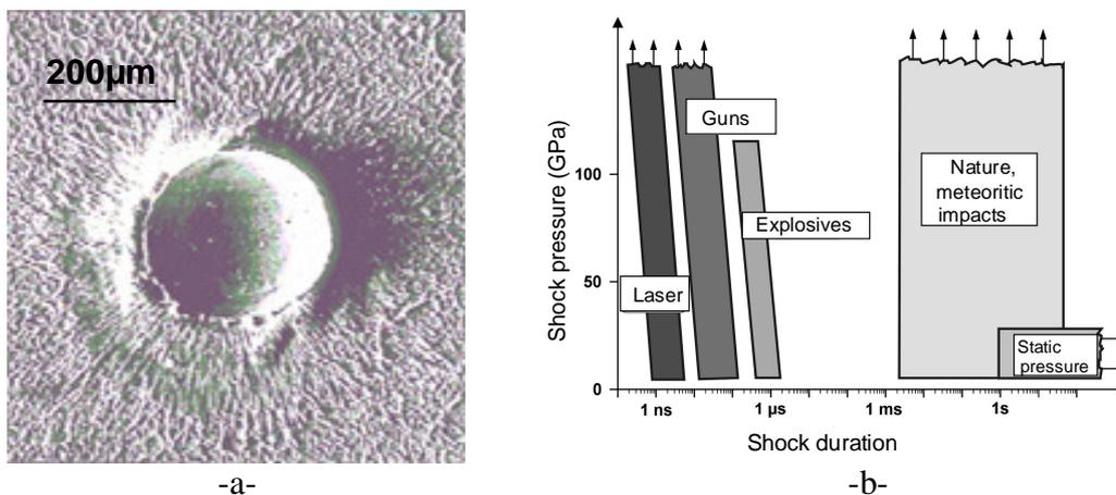
Figure 1. a-Crater generated by laser impact at 70TW/cm<sup>2</sup>, with a duration of 25ns focused on 90µm
