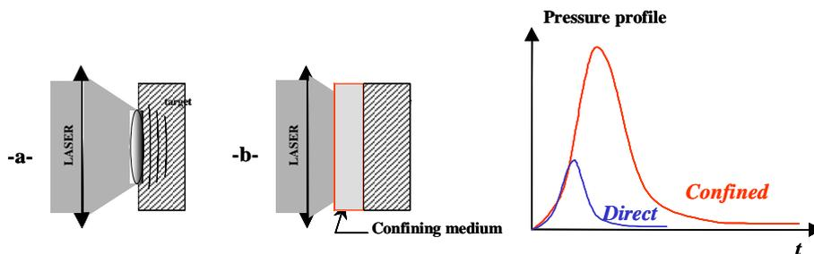
Figure 2. Shock generation in direct irradiation (a) or confined interaction (b) and associated mechanical loadings
