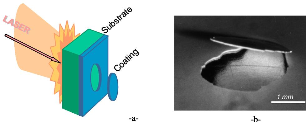
Figure 4. (a) Principle of the Laser Adhesion Test, (b) debonding of a painting  $45\mu\text{m}$  thick on aluminum substrate  $1\text{mm}$  thick by laser shock of the aluminum
