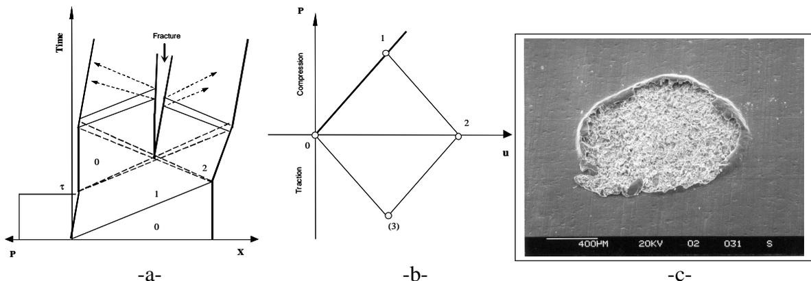
Figure 3. Principle of traction generation by shock loading of a target
