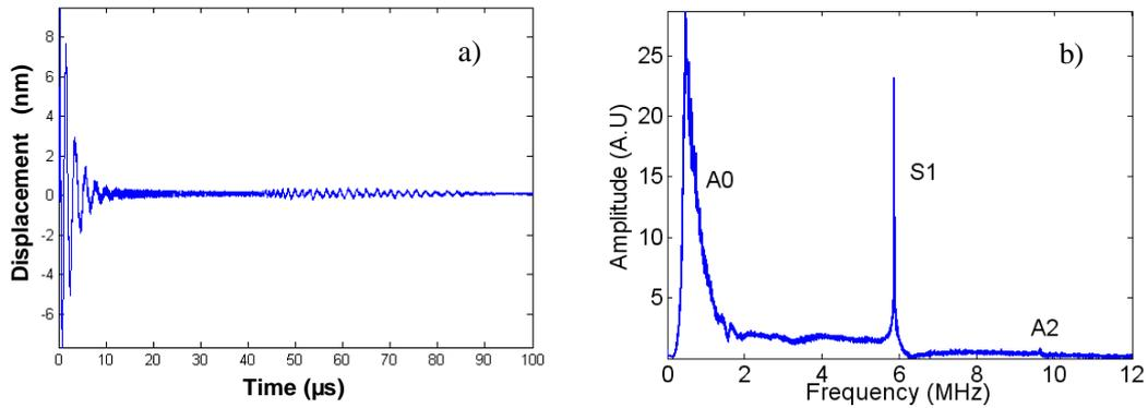
Figure 3. (a) Normal displacement and (b) spectrum generated by the absorption of the YAG-laser pulse on a 0.49-mm-thick Duralumin plate and detected at the same point by an optical heterodyne interferometer.
