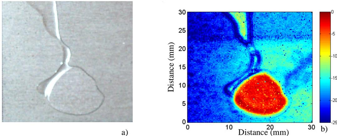
Figure 5. (a) Photography of disbond area ; (b) Amplitude (in dB) of  $S_1$ -ZGV Lamb mode.
