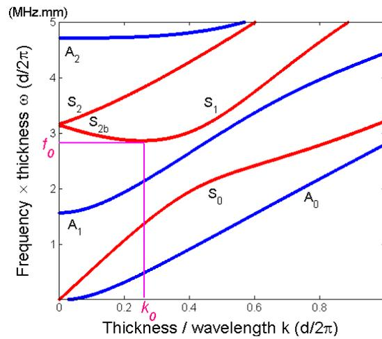
Figure 1. Dispersion curves for a Duralumin plate of thickness  $d$  and bulk wave velocities equal to  $V_L = 6.34$  km/s and  $V_T = 3.14$  km/s. Vertical scale:  $fd = \omega d/2\pi$ , horizontal scale:  $d/\lambda = kd/2\pi$ .
