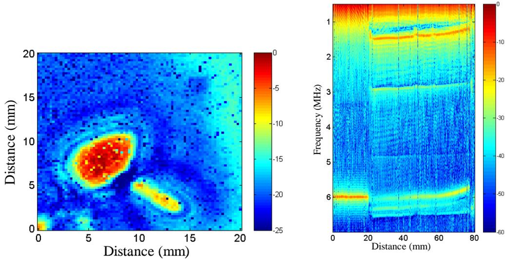
Figure 6. (a) Amplitude (in dB) of  $S_1$ -ZGV Lamb mode for two 0.5-mm thick Duralumin plates rigidly bonded and (b) Spatial Fourier transform (in dB) with variable thickness glue (0.5-mm thick Duralumin and 1.08-mm thick glass plates).
