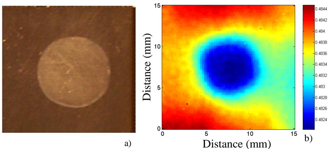
Figure 4. (a) Photograph of corroded area ; (b) thickness  $d$  (mm) of  $S_1$ -ZGV Lamb mode.
