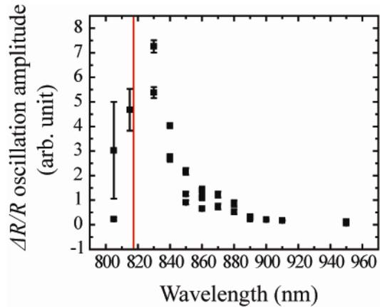
Figure 2. CAP oscillation amplitudes of CdTe measured using the two-color pump-probe spectroscopy. The red line indicates  $E_g$  of CdTe.
