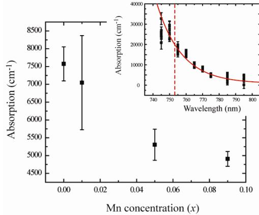
Figure 4. Absorption coefficient measured using single-color pump-probe spectroscopy at  $0.97E_g$  for various Mn concentrations. The inset shows the wavelength dependence of  $\alpha$  for  $x = 0.09$ . The red line an exponential fit serving as a guide to the eye. The dotted line indicates  $E_g = 1.65$  eV ( $\lambda_g = 753$  nm)..
