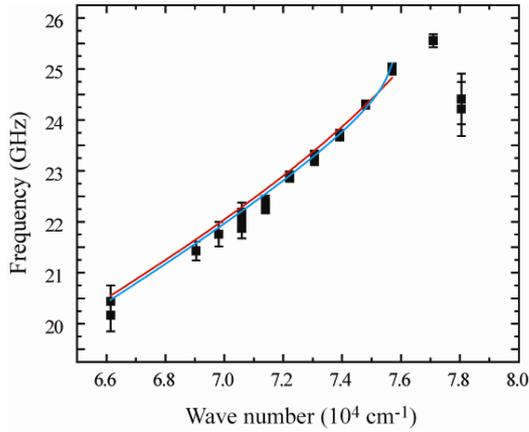
Figure 3. Dispersion curve for CdTe at room-temperature. (Red) Fitting using Schubert's equation for  $n(x)$ . (Blue) Fitting using Sellmeier's formula for  $n(T)$ .
