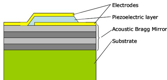
Figure 3. Cross section of an SMR-type resonator. The piezoelectric sandwich is at the top, then the acoustic Bragg mirror consisting on alternating layers of high and low acoustic impedance, and the substrate.
