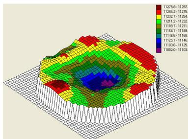
Figure 5. Typical thickness dispersion of an AlN layer (angströms).
