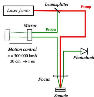
Figure 2. Schematic diagram of the experimental setup
