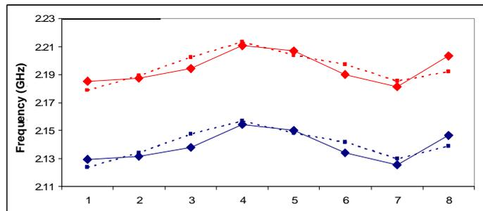
Figure 6. Measured (dotted) and simulated (line) resonant frequencies:  $f_r$  in blue and  $f_a$  in red, of a series of resonators (1 to 8) on a 200mm wafer ( $f_a$  is an anti-resonance, at this frequency the resonator can be considered as an open circuit).
