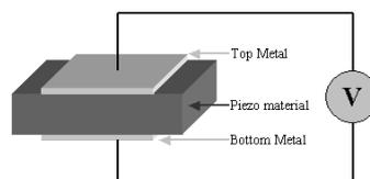
Figure 1. BAW resonator basic structure: a piezoelectric layer sandwiched between two electrodes
