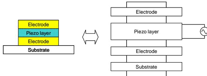
Figure 4. Electric model of a BAW resonator. On the left a BAW structure, on the right its equivalent circuit. Each layer is represented by a quadripole depending on the layers' parameters.
