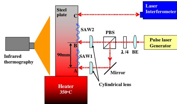
Figure 2. Schematic of the laser ultrasonic system used for monitoring SAWs of a steel being heated.
