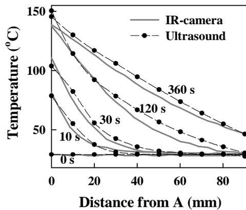
Figure 4. Comparison between temperature distributions determined by the proposed ultrasonic method and using an infrared camera.
