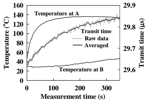
Figure 3. Variations of the temperatures and the transit time of the SAW on the steel surface during heating.
