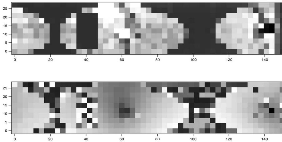
Figure 2. Through transmission C-scans of Sample A3 based on amplitude (top) and time-of-flight (bottom). Step size=3 mm.
