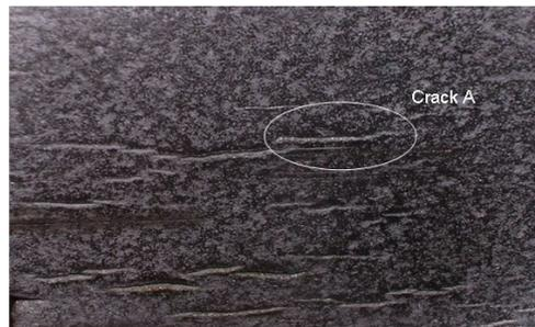
Figure 4. Photo of portion of SCC colony, showing crack that was scanned.
