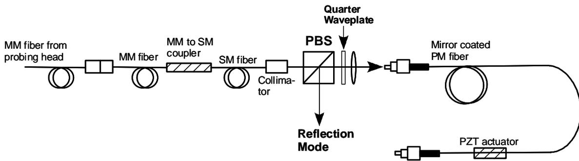
Figure 1. Detection scheme using a fiber Fabry-Perot interferometer
