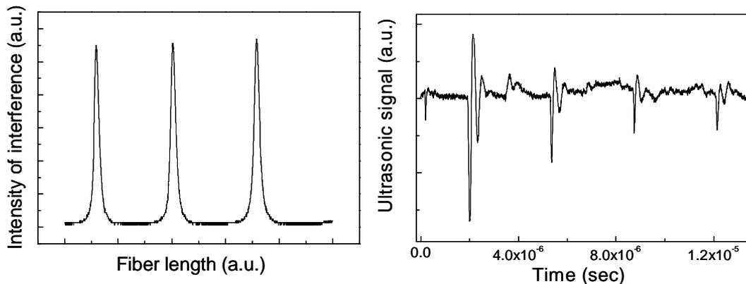
Figure 4. (a) fringe pattern of FFPI and (b) ultrasonic signals measured by FFPI with 3 m cavity length
