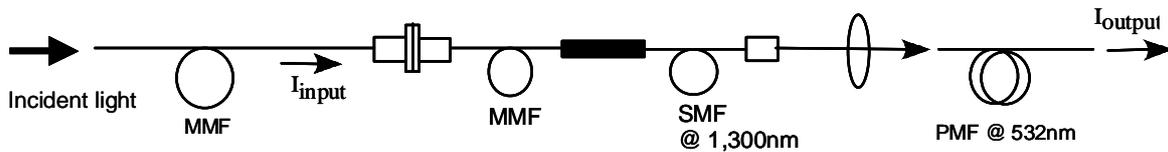
Figure 2. Evaluation of coupling efficiency from MMF to PMF
