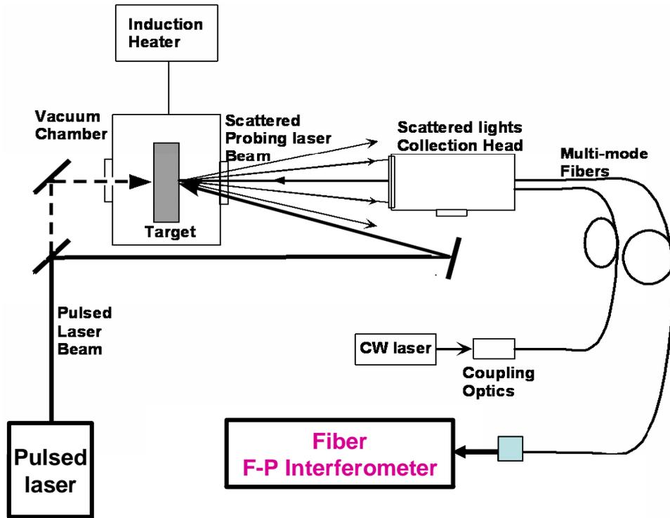
Figure 3. Experimental setup for generation and detection of laser-ultrasound
