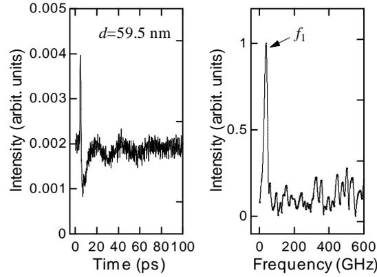
Figure 1. Typical phonon oscillation observed by the picosecond-laser ultrasounds (left), and the corresponding Fourier spectrum (right).
