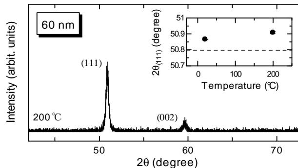
Figure 3. X-ray diffraction spectrum of the Cu thin film annealed at 200 °C. An inset shows the diffraction angle from (111) planes, and the broken line is the diffraction angle of bulk Cu.
