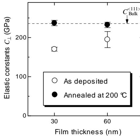
Figure 4. Elastic constants of Cu thin films. The broken line indicates the elastic constant governing the velocity of the longitudinal wave that propagates in the  $\langle 111 \rangle$  direction of Cu.
