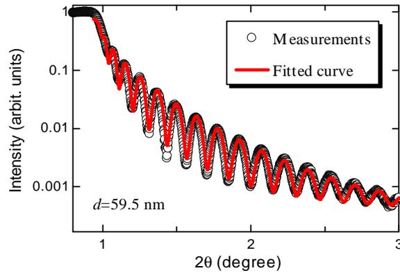
Figure 2. X-ray reflectivity spectrum of the Cu film. Open circles and a line indicate the measured and fitted reflectivity spectrum, respectively.  $\text{CoK}\alpha$  x-ray source was used.
