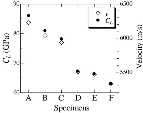
Figure 4. Elastic constant and sound velocity of  $\alpha$ -SiO<sub>2</sub> thin films.
