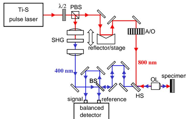
Figure 1. Optics for the pump-probe detection of Brillouin oscillations.
