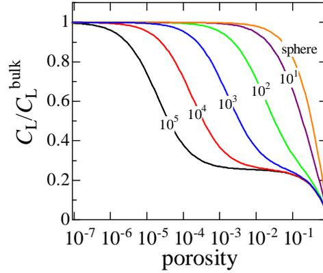
Figure 5. Change in the elastic constant  $C_L$  caused by defects. The numbers denote the aspect ratio of the defect.
