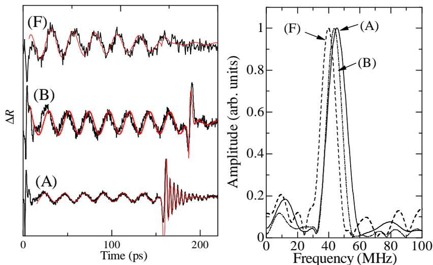
Figure 3. Measured (black lines) and calculated (red lines) reflectivity changes of specimens A, B, and F (left), and their corresponding Fourier spectra (right).
