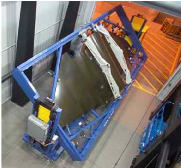
Figure 6. Large Part Inspected on Transportation Tool
