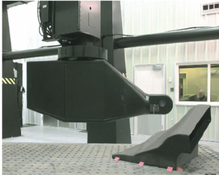
Figure 1. Beta LaserUT System Inspecting F22 Duct Section
