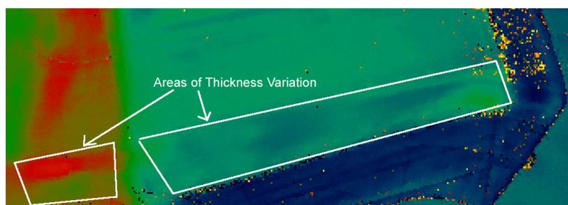
Figure 2. Thickness Map of Lower Radius
