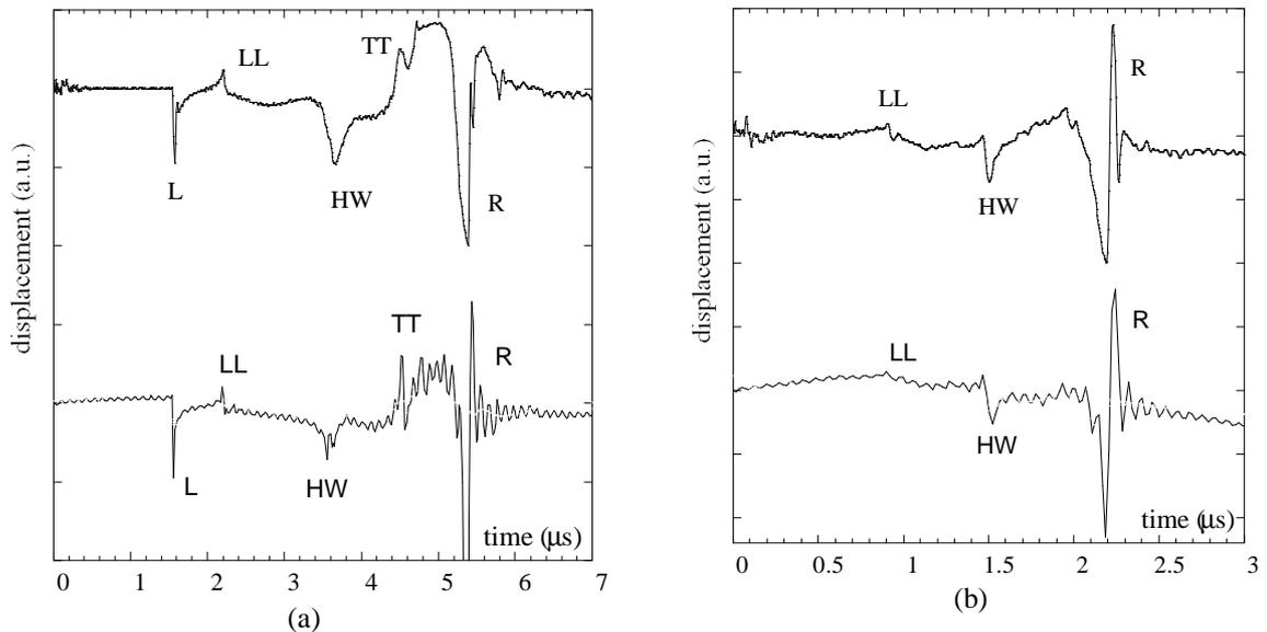
Figure 1. Experimental (top) and calculated (below) displacements at an observation angle of  $180^\circ$  for an aluminum cylindrical rod under (a) ablation regime (b) thermoelastic regime.
