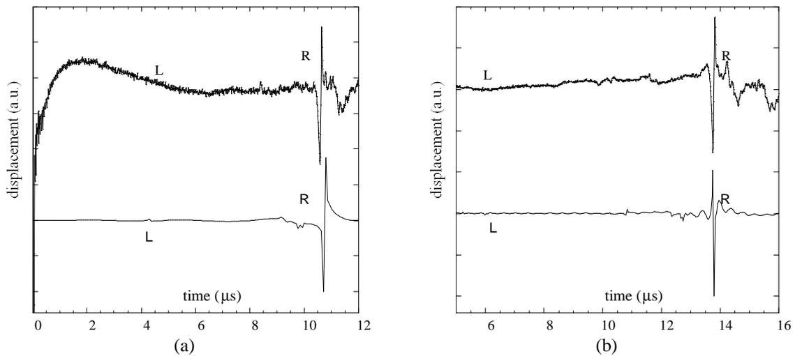
Figure 3. Experimental (top) and calculated (below) displacements for an aluminum cylindrical cavity at an observation angle of (a)  $90^\circ$  (b)  $115^\circ$ .
