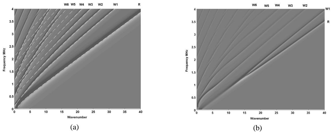
Figure 2. Dispersion spectrums for (a) cylindrical rod and (b) cylindrical cavity.
