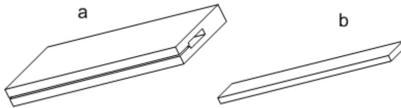
Figure 3. Specimen a) was tested with LUS. Specimen b) for dynamic mechanical analysis was extracted after LUS measurements.
