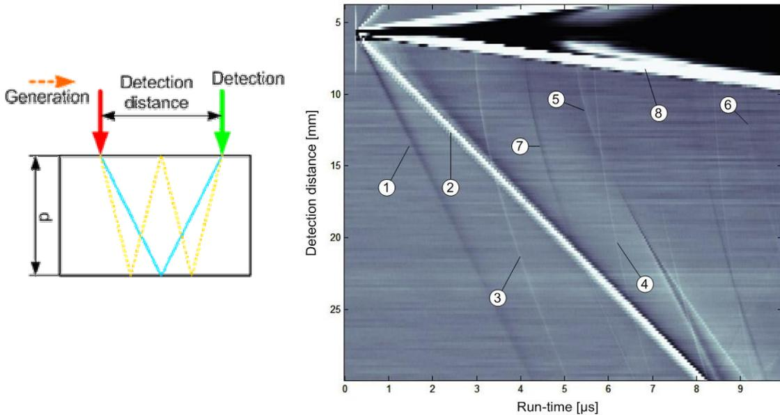
Figure 1. Measurement Setup. During measurement the generation was moved along the surface towards the detection point. The yellow and blue lines mark the first and second echoes of bulk waves.
