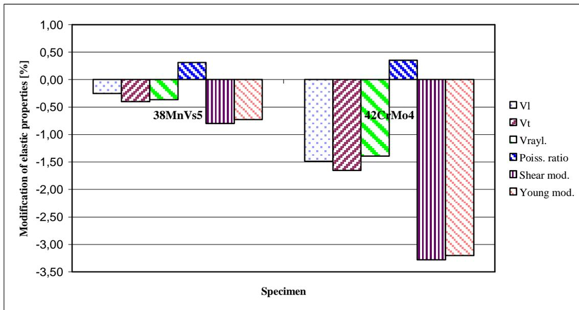
Figure 4. Alteration of the elastic properties by hardening, measured with Laser-Ultrasonic-Setup.
