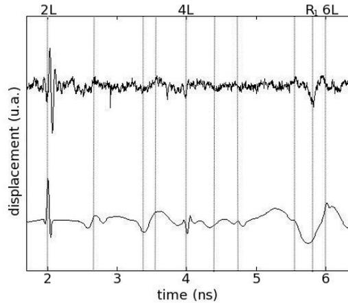
Figure 1. Comparison between experimental signal (top) and theoretical displacement (bottom) on a tungsten fibre of  $5 \mu\text{m}$  diameter. The thermal background was removed from the experimental data
