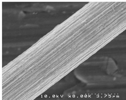
Figure 2. Photograph of a tungsten fiber with a micrometer diameter, captured by the Scanning Electron Microscopy
