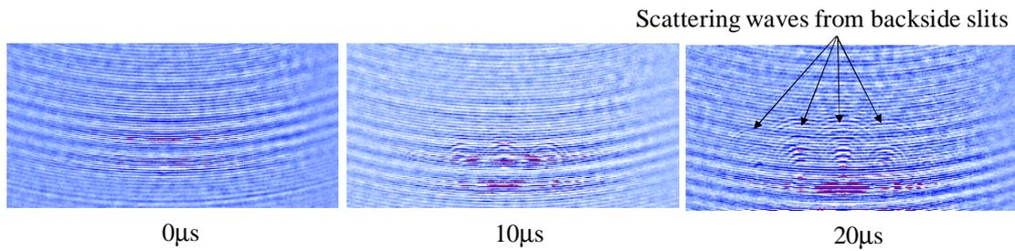
Figure 7. Ultrasonic propagation image of an aluminum plate with rear slits
