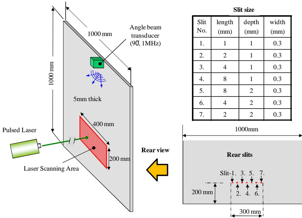
Figure 6. Experimental setup for visualizing ultrasonic waves propagating on an aluminum plate with some slits on its rear surface
