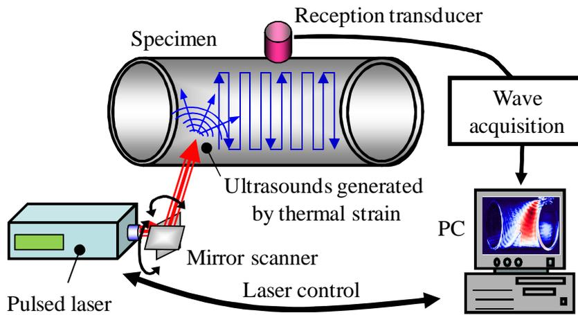
Figure 1. Schematic of the generation laser scanning method
