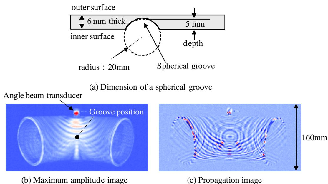
Figure 5. Ultrasonic propagation image of a stainless steel elbow pipe
