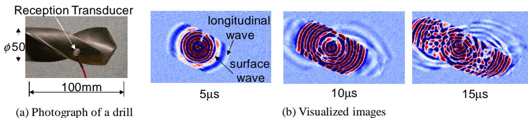
Figure 4. Visualization of an ultrasonic wave propagating on a drill blade.
