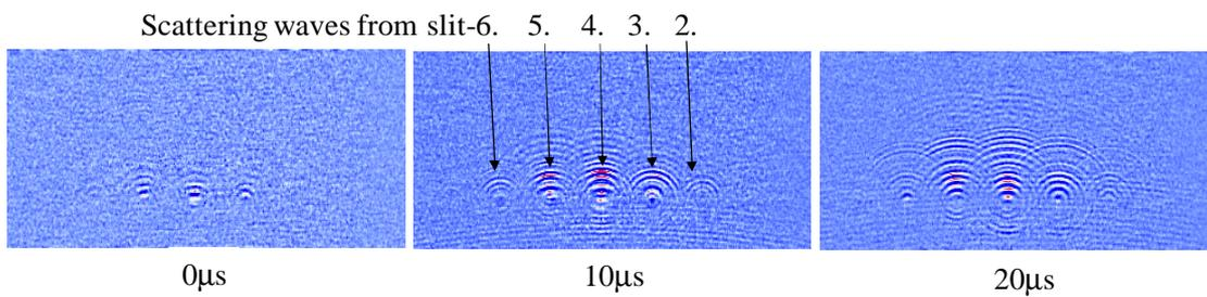
Figure 8. Ultrasonic propagation image of an aluminum plate with rear slits after data processing
