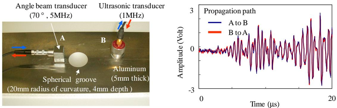
Figure 2. Reciprocity of wave propagation between transmission and reception PZT transducers.
