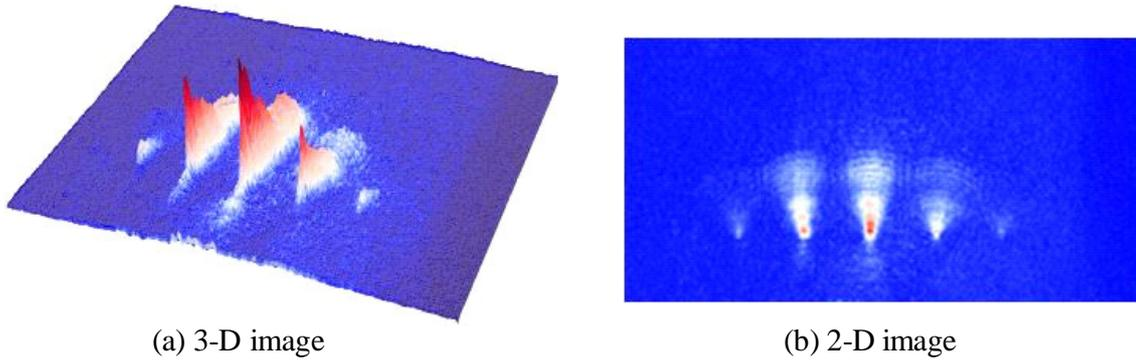
Figure 9. Maximum amplitude image of scattered waves from rear slits after data processing
