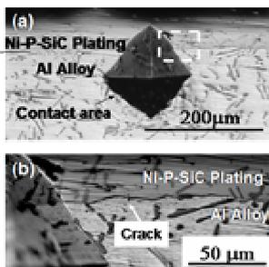
Figure 9 Micrograph of contact region for Ni-P-SiC / Al alloy using a Vickers indenter
