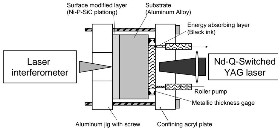
Figure 1 Experimental setup for laser spallation method
