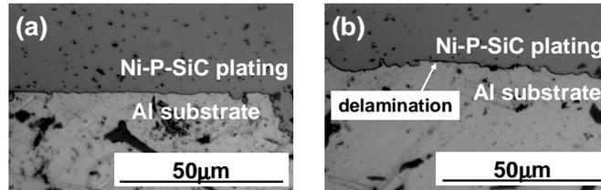
Figure 5 Cross-sectional images after laser spallation test at laser energy of (a) 35 mJ and (b) 37.5 mJ
