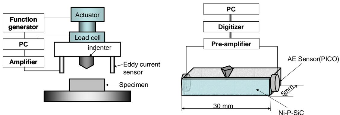
Figure 6 Experimental setup for indentation testing
