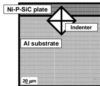
Fig.10 Top view of three dimensional FEM model for Ni-P-SiC / Al alloy
