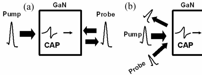
Figure 1. Schematic diagram of (a) two-sides and (b) one-side pump-probe CAP experiment.
