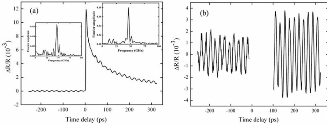
Figure 3.  $\Delta R/R$  signal obtained using two-color pump-probe spectroscopy. (a) Full time-resolved  $\Delta R/R$  transient. The insets in (a) are fast Fourier transforms (FFTs) of the oscillation before and after the zero-delay, respectively. Both have the same peak frequency at 46.3 GHz. (b) Two CAP oscillations corresponding to signals before and after the zero-delay point.
