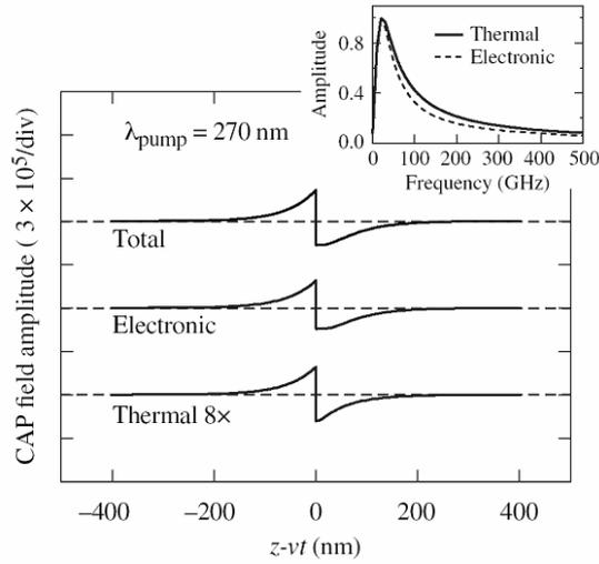
Figure 2. Simulation of spatial-time profiles of propagating CAP transients generated by the electronic stress, thermal stress, and both, respectively. The CAP pulse was excited by the pump beam with the photon energy of 4.59 eV. The inset shows the frequency spectra of the electronically (solid line) and thermal induced (dashed line) CAPs.
