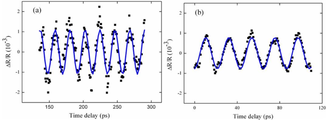
Figure 4.  $\Delta R/R$  signal obtained using two-side pump-probe spectroscopy. (a) CAP oscillations (dots) within a 200-ps time window. (b) CAP oscillations measured after 13 ns time delay at the end surface of the crystal. The solid lines in (a) and (b) represent the fits based on Eq. (2).
