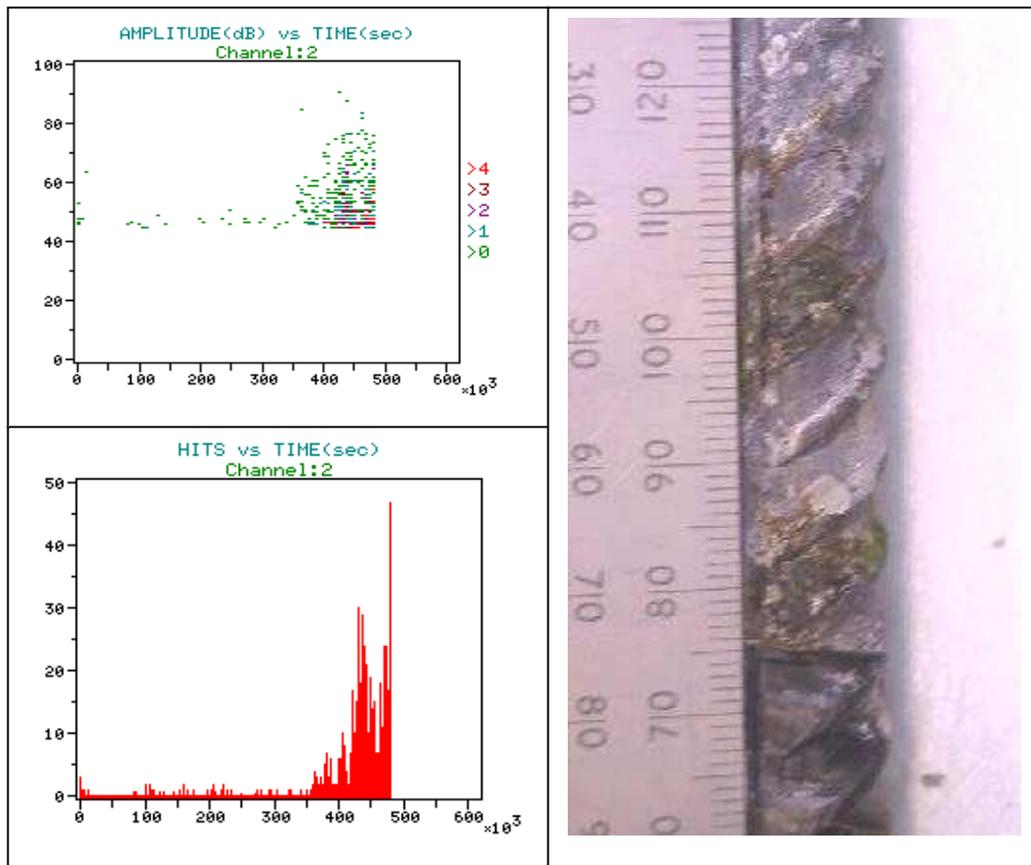
Figure 5: Onset of propagation detected by AE monitoring, and corresponding damage after break-out.
