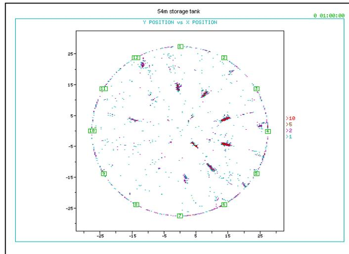
Figure 2: 2D Location analysis from a tank floor test showing emission from sacrificial zinc anodes (red).
