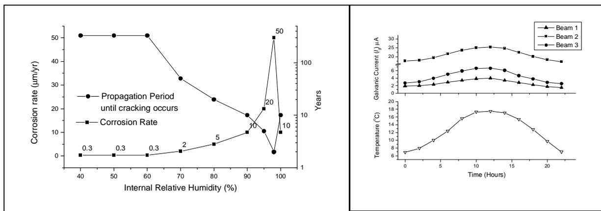
Figure 4: Effect of internal humidity and temperature on corrosion rate.
