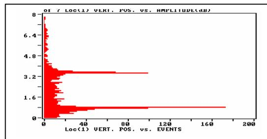
Figure 3: Vertical distribution of emission from a tank shell, concentrations are at insulation support rings.
