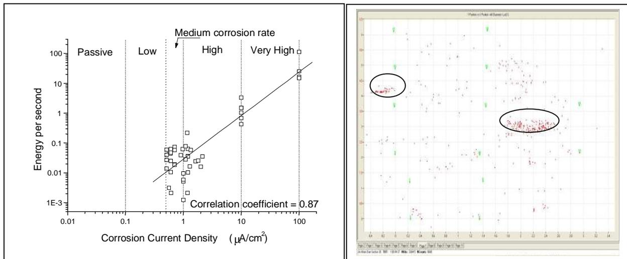
Figure 6: Corrosion current density versus emission energy rate, damage located in a concrete structure.
