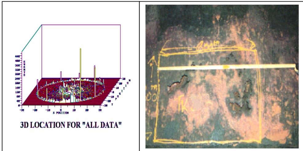
Figure 1: 3D Location analysis from a tank floor test using acoustic emission, and internal damage.
