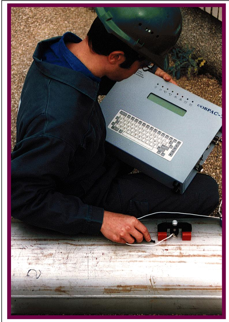
Figure 8: Corrosion monitoring using the Mark 1 CORPAC system.
