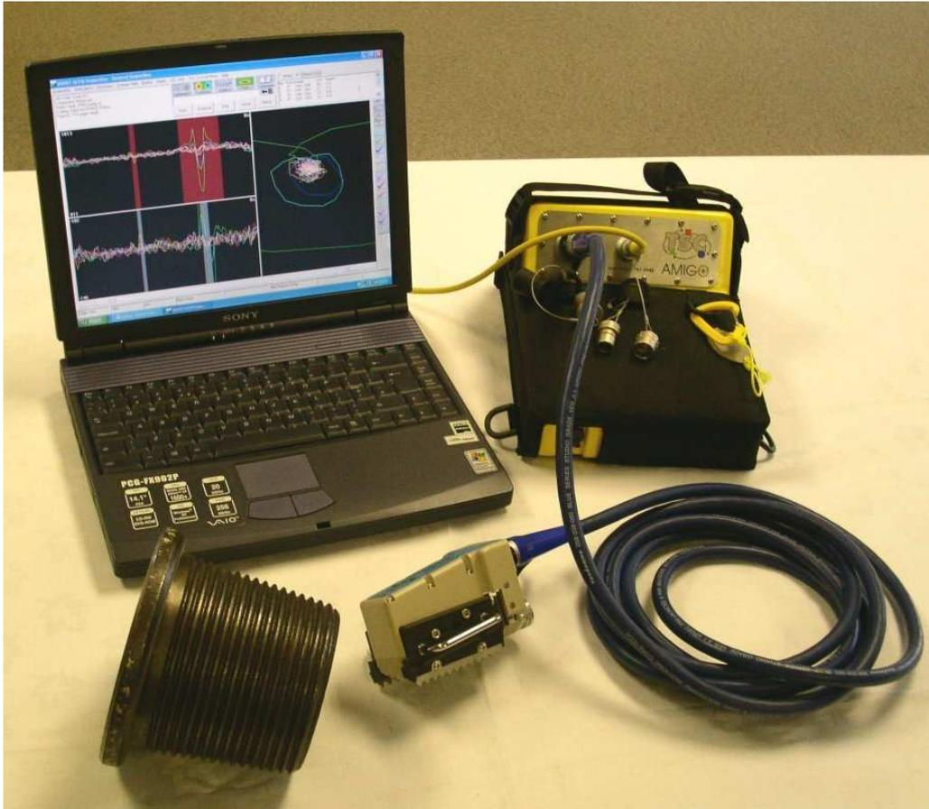
Figure 4. ATI system showing PC, Amigo instrument and 4 tpi array probe
