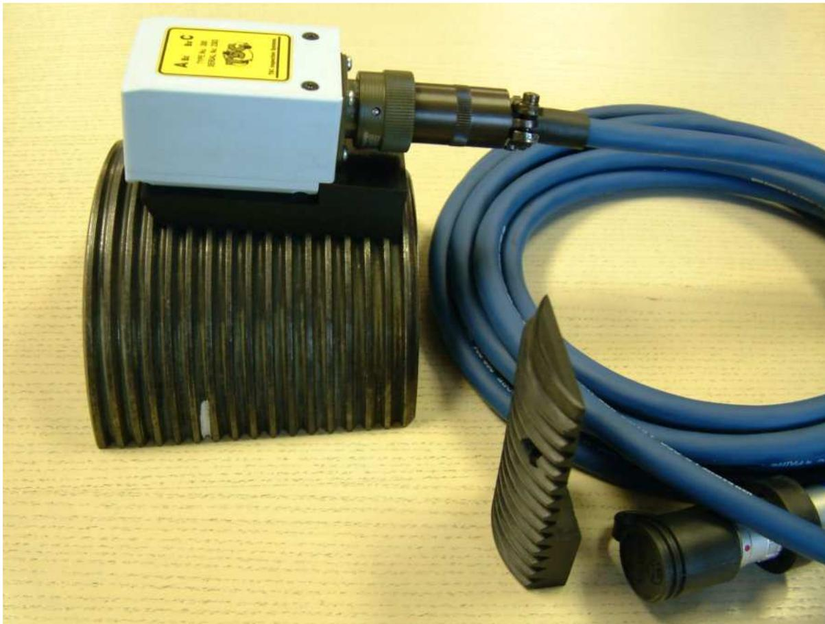
Figure 3. Simple thread probe deployed on pin, and shoe for box
