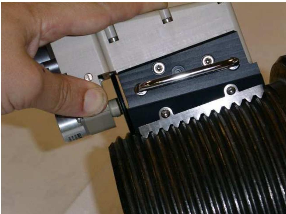
Figure 5. ATI probe set up for pin inspection
