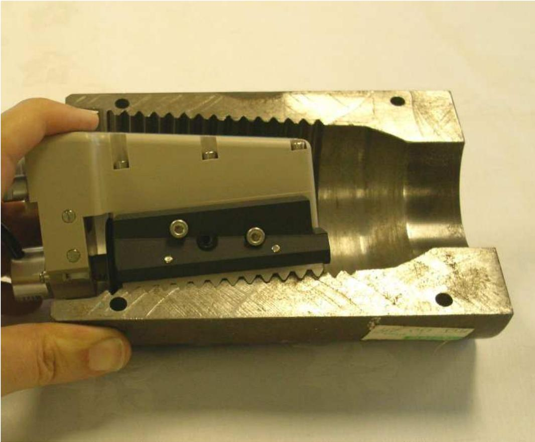
Figure 6. ATI probe set up for box inspection
