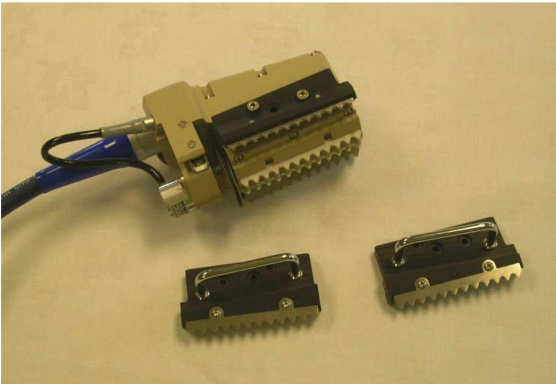
Figure 7. ATI probe with 4.5" 4tpi scrapers for box (fitted) and pin
