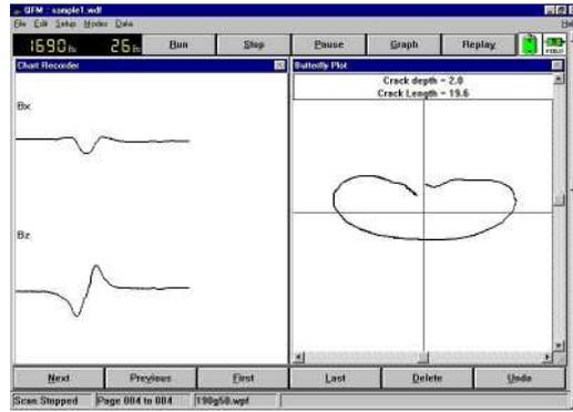
Figure 2. Typical ACFM data from a crack, with butterfly plot on right
