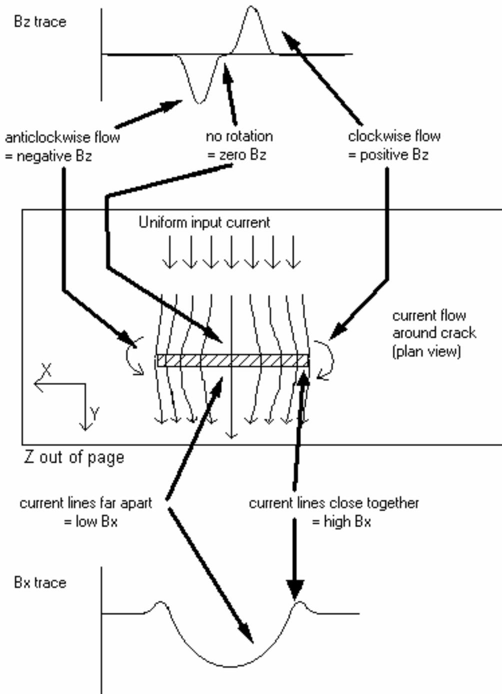
Figure 1. Current Flow and a surface breaking defect
