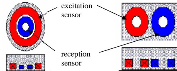
Figure1. Diagram of the probes used one controls by PEC
