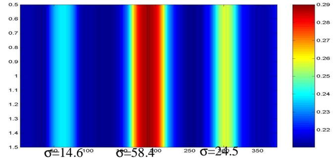
Figure 8b. Representation of inclusion defect simulated by three type of conductivity
