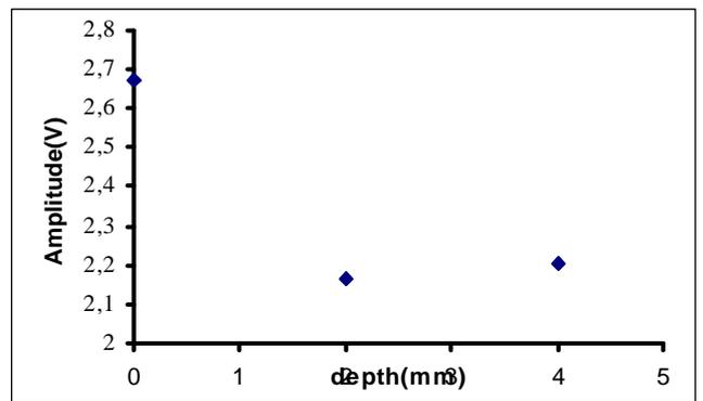
Figure5b. Variation of amplitude according to the defect depth
