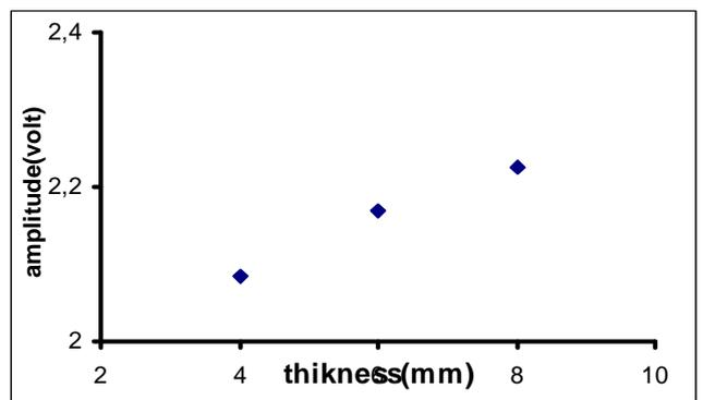
Figure6b. Amplitude variation of defect on 2<sup>nd</sup> layer according to thickness
