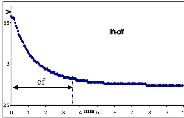
Figure4. Variation of amplitude with Lift off
