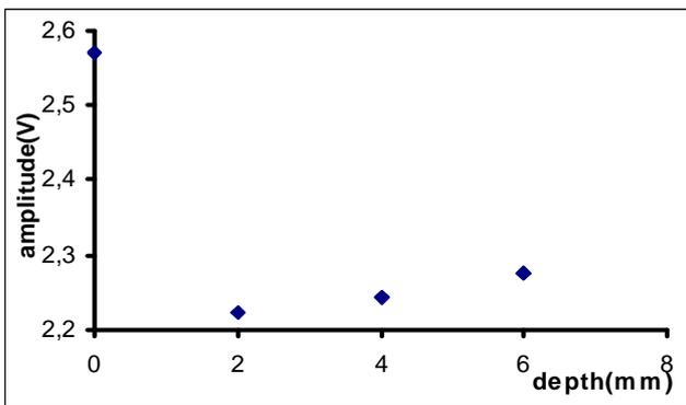
Figure5a. Variation of the amplitude in function defect depth
