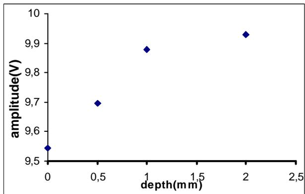
Figure7a. Variation of defect depth for 31A008
