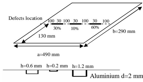
**Figure 5: The schematic mapping of fabricated Aluminum plate**
