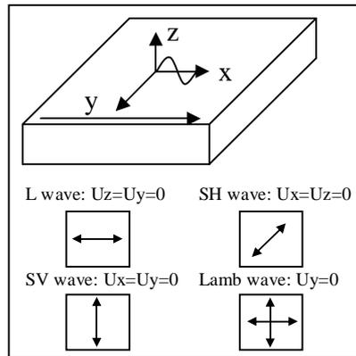
**Figure 1: Schematic illustration of ultrasonic wave modes**
