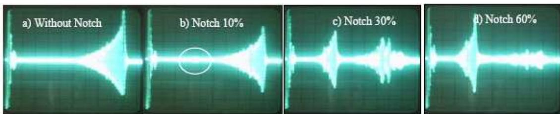
**Figure 8: The waveforms of ultrasonic lamb wave in pulse-echo technique,  $a_1$  mode evaluated (defect to probe distance was 75 mm)**
