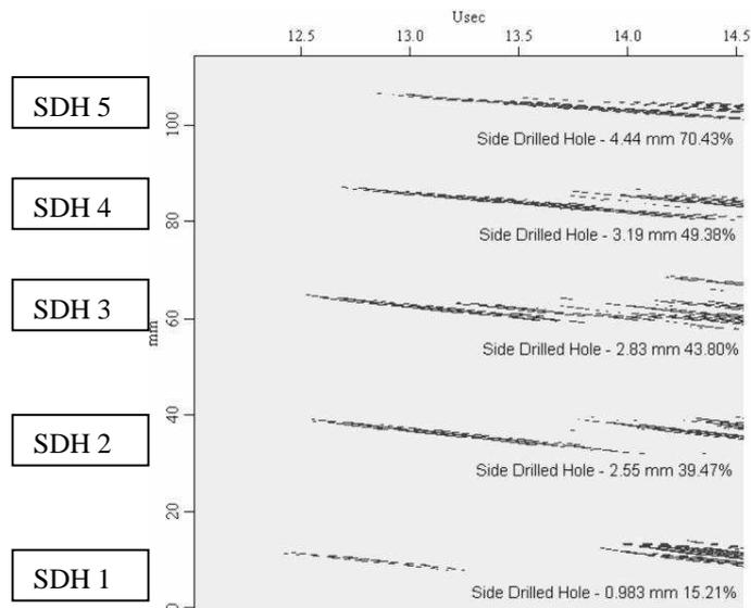
Figure 13: B-Scan of Calibration SDH
