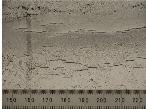
Figure 8: Typical Low pH SCC Colony
