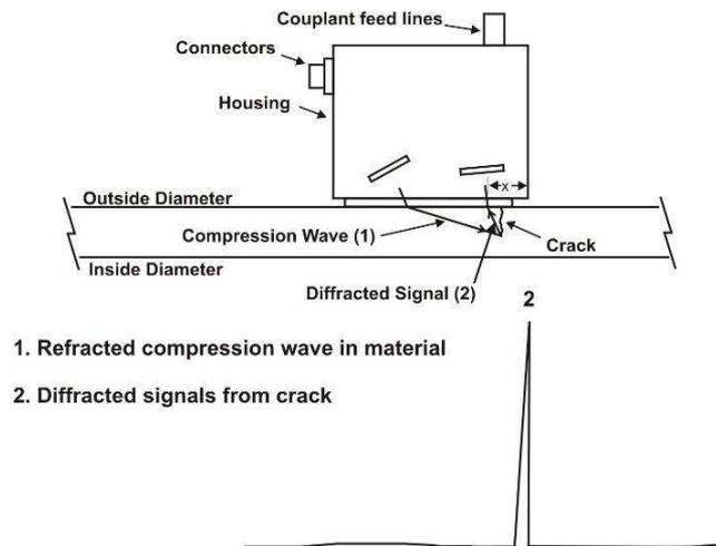
Figure 10: NSDS Transducer
