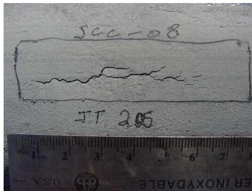
Figure 9: Typical High pH SCC Colony
