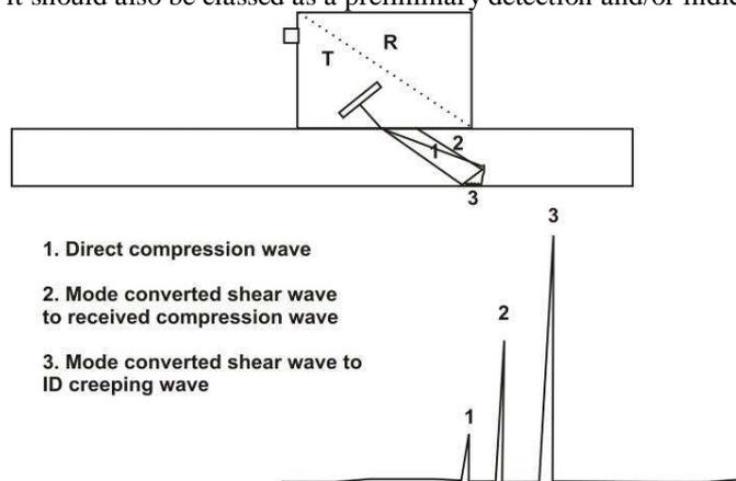
**Figure 4: Typical Creeping Wave Transducer with Signal components**
