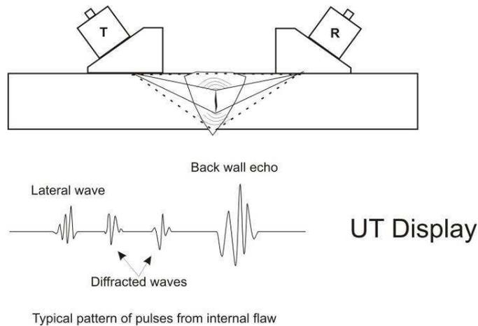
**Figure 5: TOFD (Delta) Transducer Arrangement**
