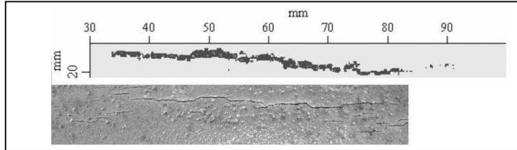
**Figure 16: C-Scan of SCC indication**
