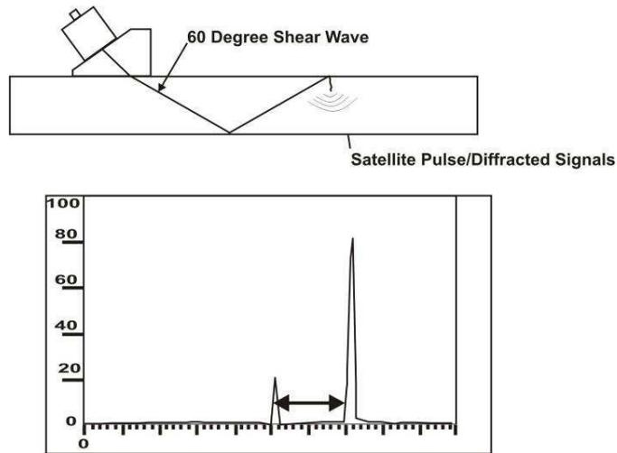
Figure 6: Illustration of Satellite Pulse Techniques SPT
