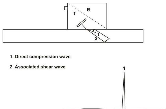
**Figure 2: High Angle Longitudinal Wave Technique**
