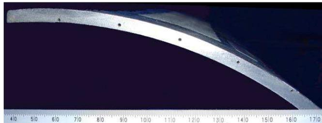
Figure 14: Calibration Sample with Side Drilled Holes
