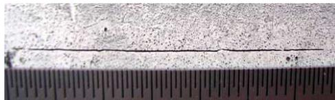
Figure 7: Linear Indication Along Electrical Resistance Weld (ERW)
