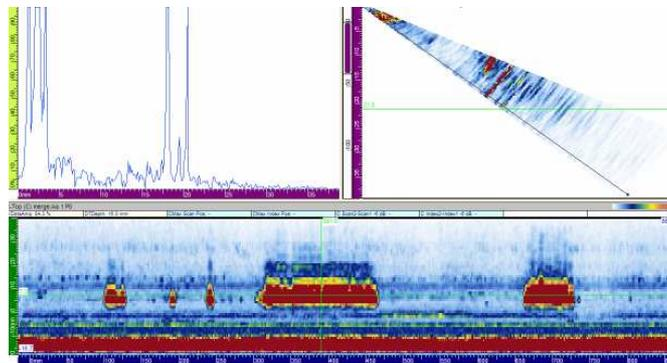
**Figure 17: Phased Array Scan of 25.4cm Diameter ERW Weld with ID Linear Indications within the ERW**
