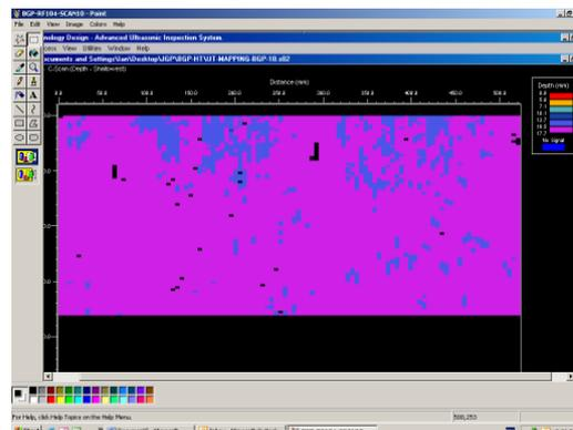
Figure 15: C-Scan showing minor wall loss.
