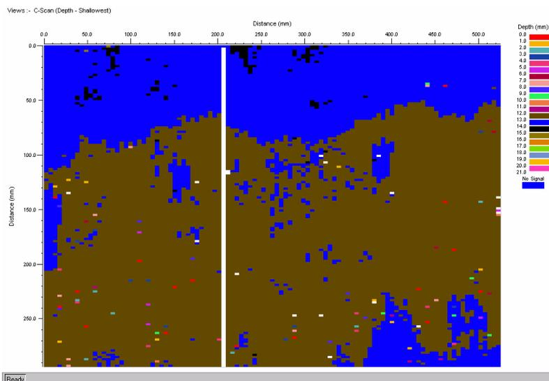
Figure 10: C-Scan showing material thickness 13mm (brown), 14mm (blue) & 15mm (black)
