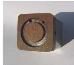
Figure 6: bottom of transducers
