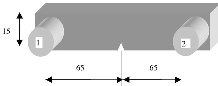
Fig.2 Pre-notched sample for test
