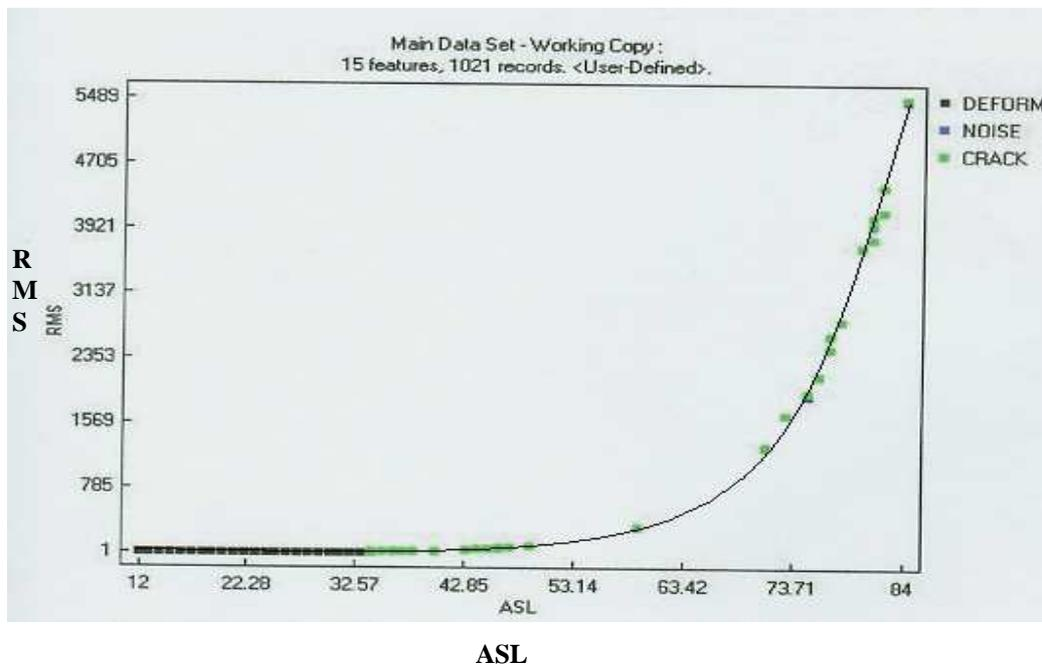
FIG.6 AE signals for complete test.
