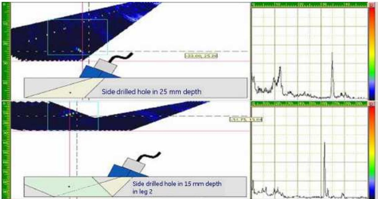
Figure 8b: Side drilled holes at depths of 5mm & 15mm (in reflection)
