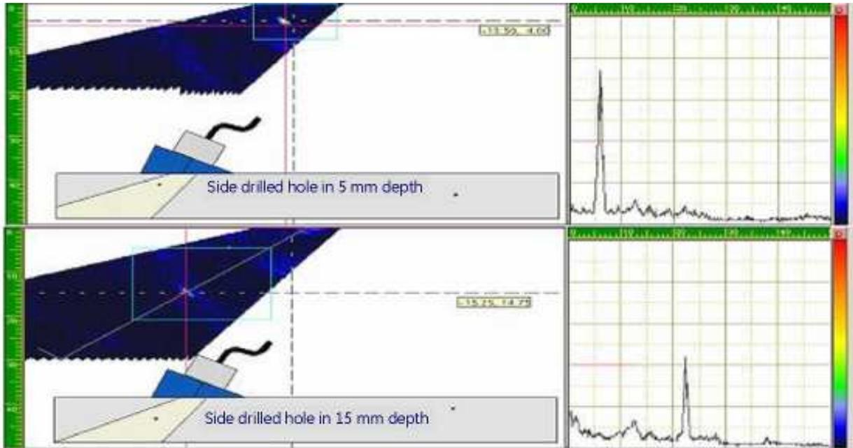
Figure 8a: Side drilled holes at a depth of 5 mm and 15mm
