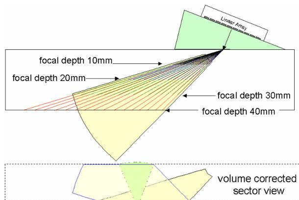
Figure 5: Sector representation with angle probe
