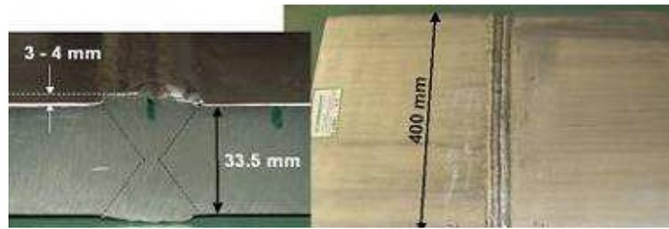
Figure 9: Weld seam
