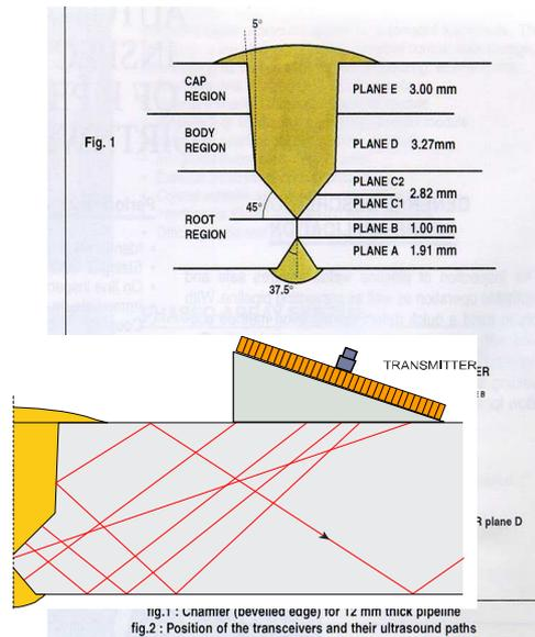
Figure 4: Schematic showing zones on a CRC-Evans weld profile, and ultrasonic beams from a phased array probe.
