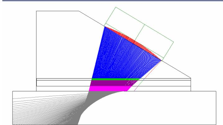
Figure 6: Imagine3D modeling of phased array and wedge on pipe, with temperature gradient in layers from base.
