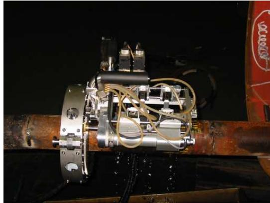
Figure 8: Small diameter scanner.
