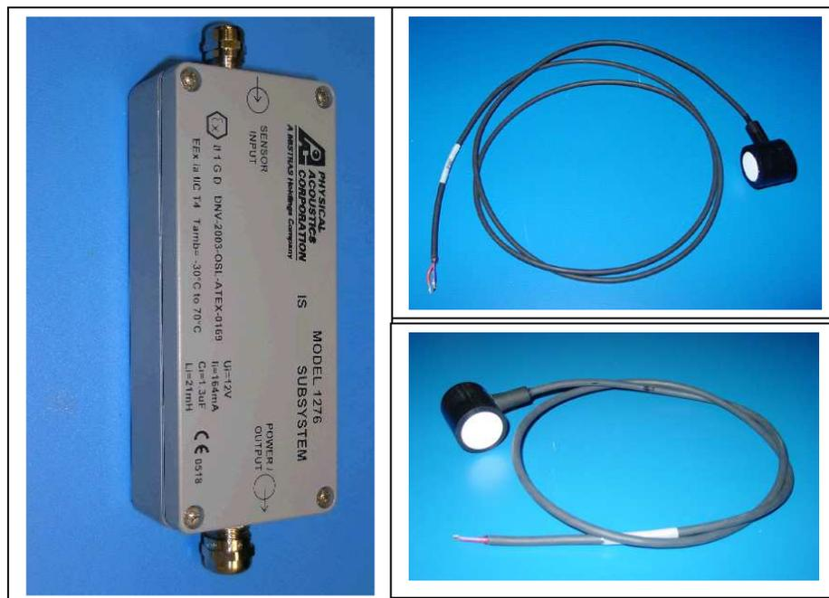
**Figure 2: Acoustic Emission sensors, I.S unit top right is used with the I.S. pre-amplifier (left), the larger sensor has a built in pre-amplifier and will drive 500m of cable, but is not I.S. certified. All are IP66 rated.**
