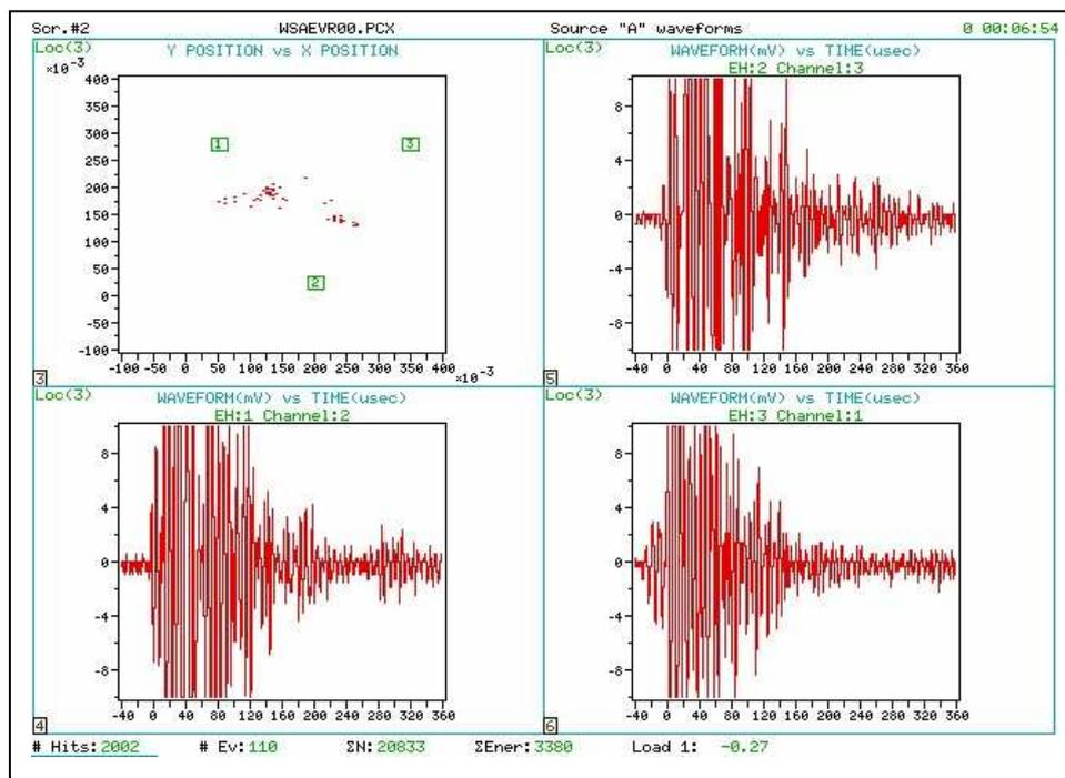
Figure 1: Acoustic Emission event signal detected at three sensors around a growing fatigue crack.
