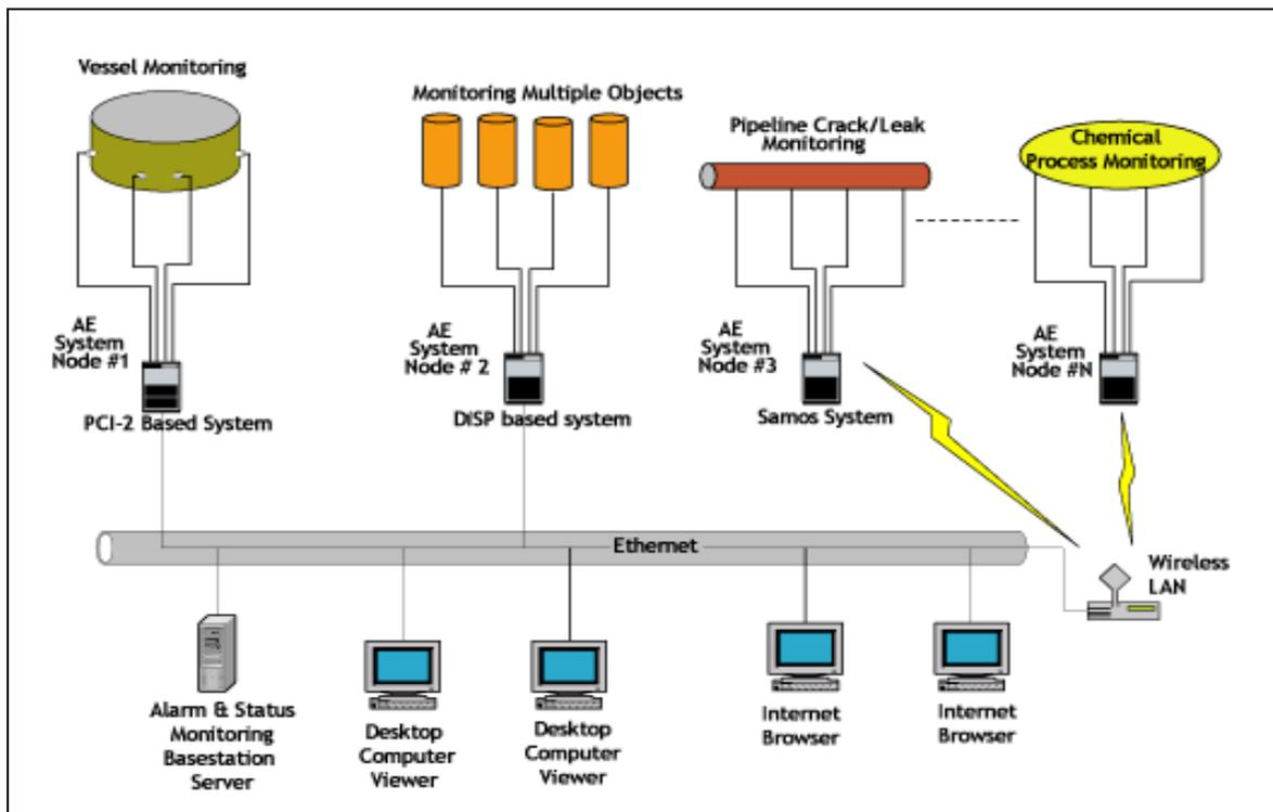
**Figure 4: Typical network of multiple networked nodes, base-station web server, expert access “viewers” that can re-configure the nodes, and any browsers which may look at the processed “web” data (with password).**
