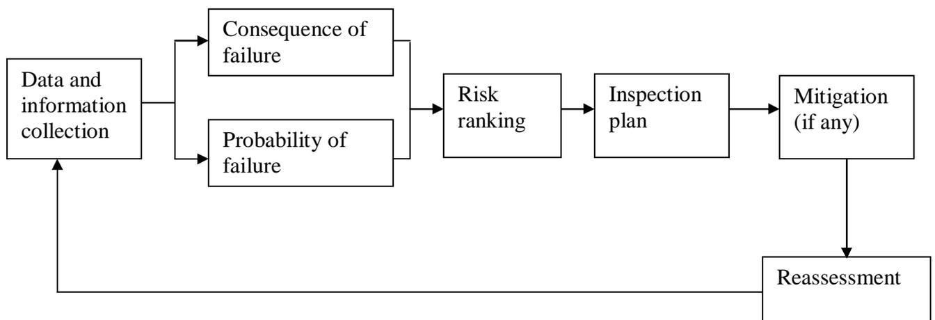
The RBI process consists of performing a risk assessment of the equipment, then determining inspection frequencies and scopes. Many types of RBI methods exist and are currently being applied throughout industry.
