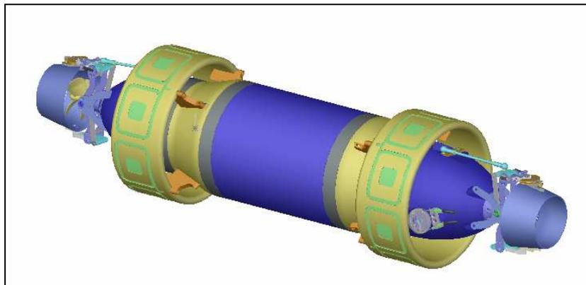
**Figure 9. *RoFloat*: Free swimming leak detection tool**
