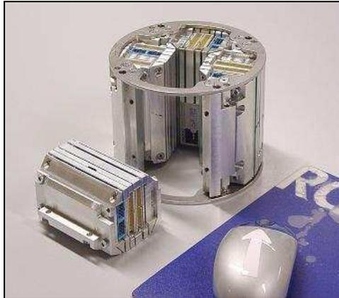
**Figure 4. Modular components for data acquisition, recording and processing (ROSEN “SMART Boxes”)**
