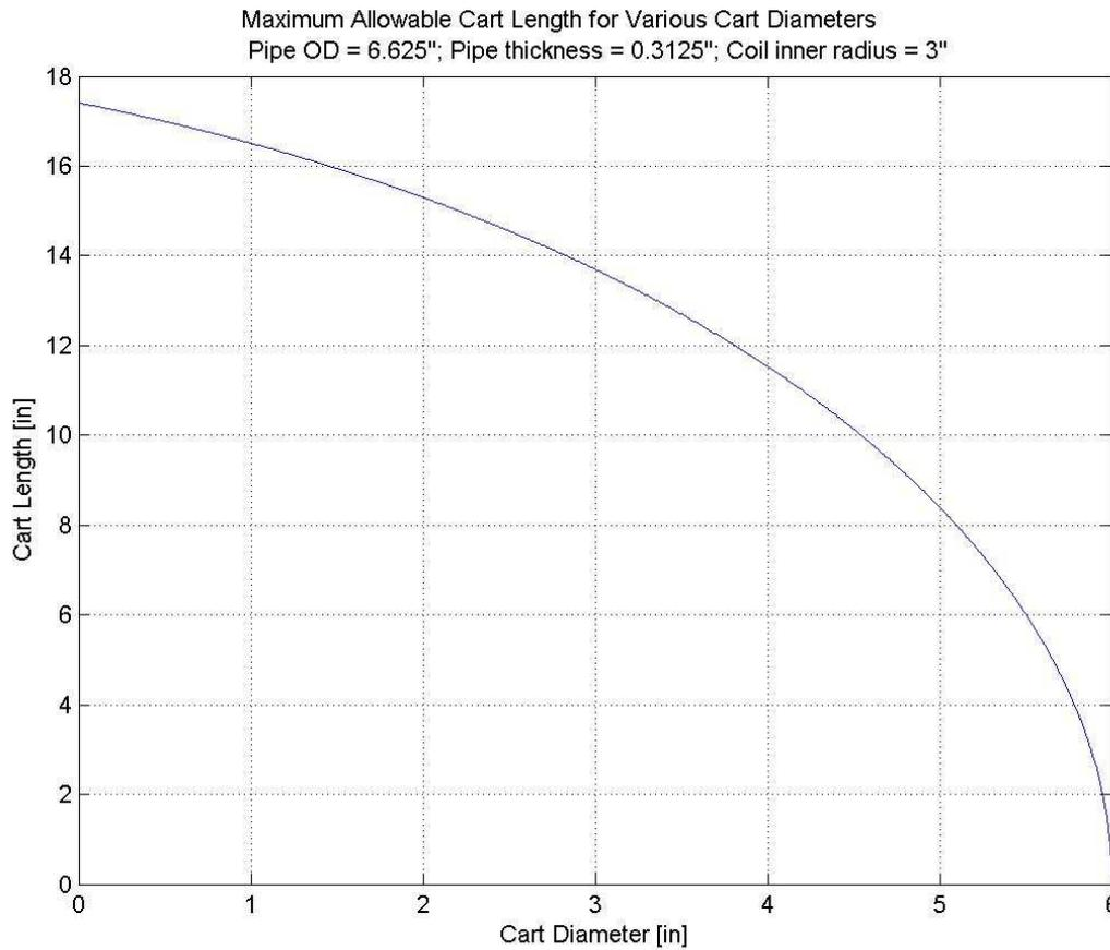
Figure 1 - Maximum Size of a Cylindrical Cart Able to Traverse a 1-D 180° Section of a 6" ID Pipe
