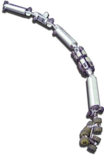
Figure 2 -- The Small Pipe Inspector (SPI)
