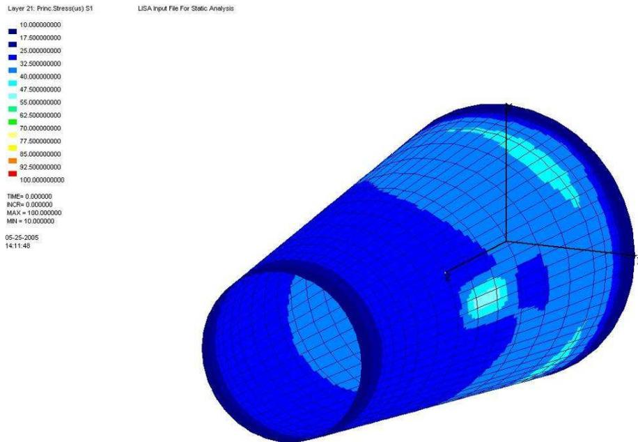
**Figure 8: Outer surface principal stress ( $\sigma_1$ ) distribution**
