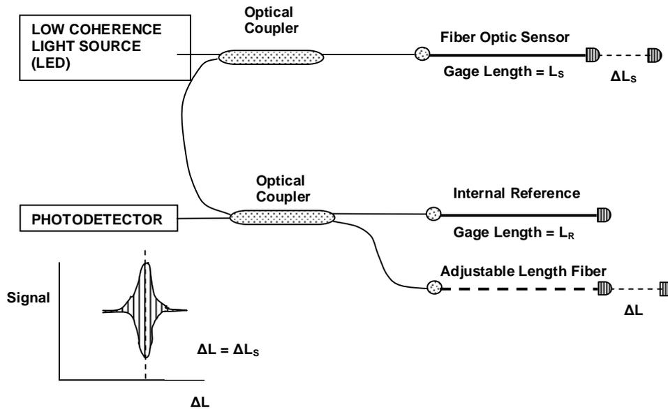
**Figure 1: FT Fiber Optic Sensor system schematic**
