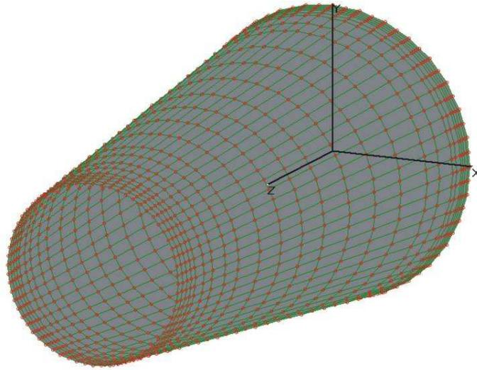
**Figure 7: Finite Element Model of Reducer with 3072 Shell Elements and 3074 Nodes**
