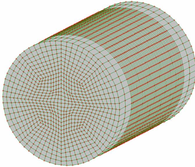
**Figure 10: Finite element model of overhead line section with 4608 shell elements**
