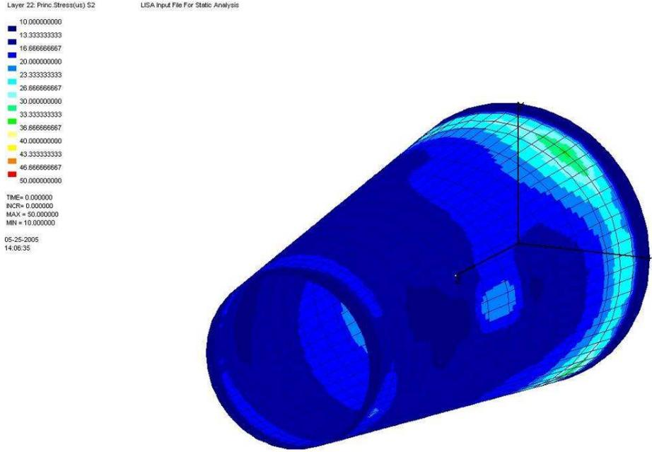
**Figure 9: Outer surface principal stress ( $\sigma_2$ ) distribution**
