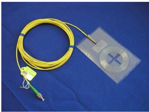
Figure 3: FT Coil Sensor for corrosion, crack, pressure, temperature
