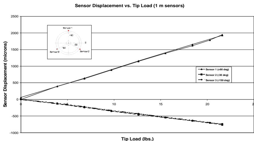
**Figure 2: Typical linear displacement-load response of FT Sensor**
