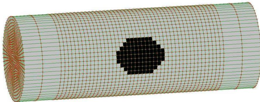
**Figure 11: Location of reduced thickness elements to simulate corroded area**
