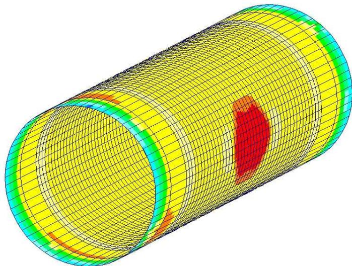
Figure 13: Principal stress ( $\sigma_2$ ) distribution in axial direction
