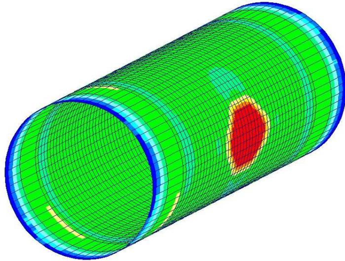
Figure 12: Principal stress ( $\sigma_1$ ) distribution in hoop direction
