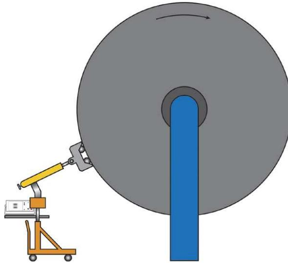
Figure 24: Rotating vessel for automated inspection.
