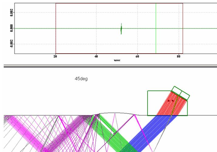
Figure 14: Imagine3D simulation of S-scan inspecting 25 mm plate with LOF midwall defect.
