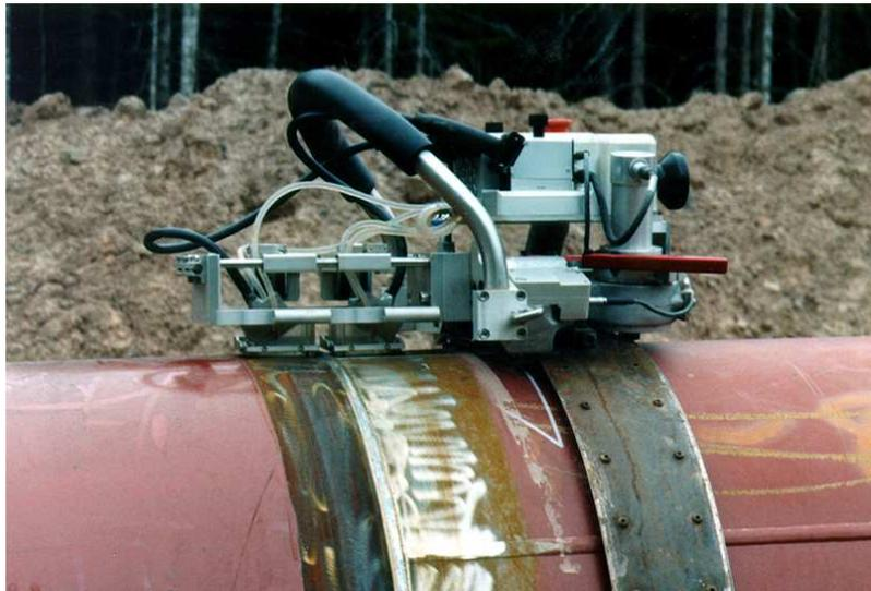
Figure 23: Pipe scanner on welding band.
