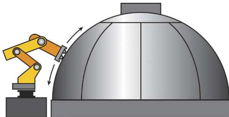
Figure 26: Schematic showing robotic scanner on curved head.
