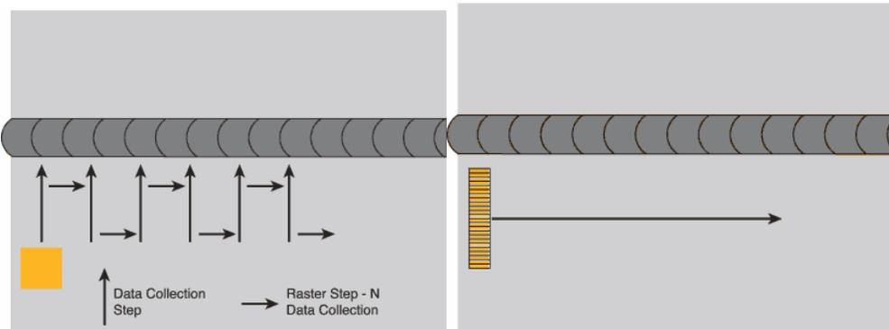
Figure 7a (left), conventional raster scanning; 7b (right), linear scanning.
