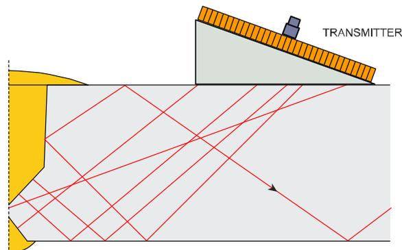
Figure 9: Schematic showing phased array performing zone discrimination.
