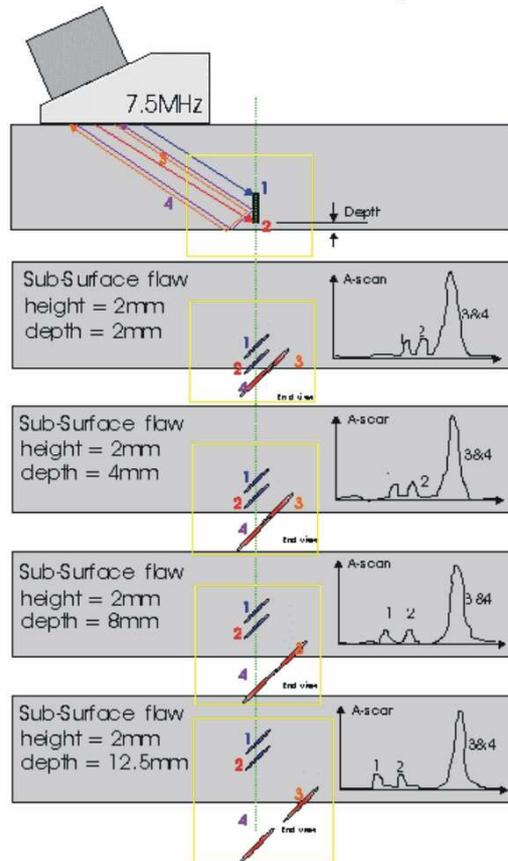
Figure 11: Schematic showing the back-diffraction concept.
