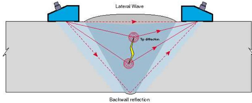
Figure 10: Schematic of TOFD set-up.
