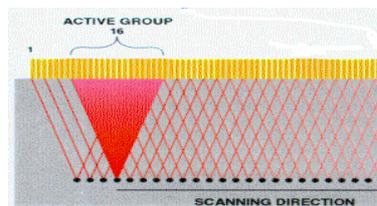
Figure 4: Schematic illustration of electronic scanning.
