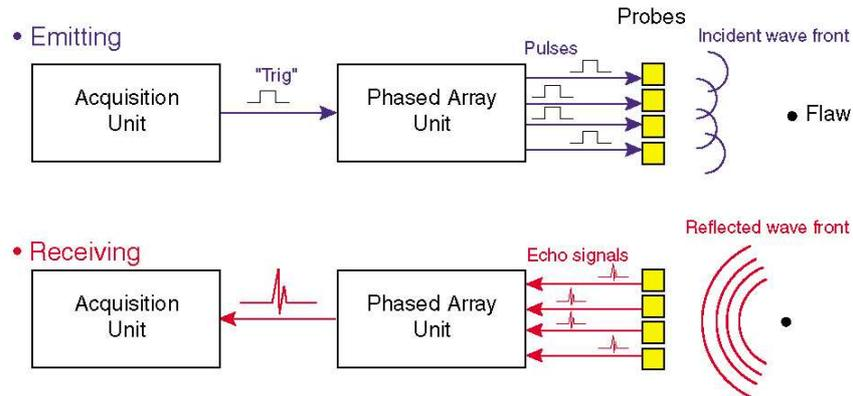
Figure 3: Beam forming (above) and receiving (below).
