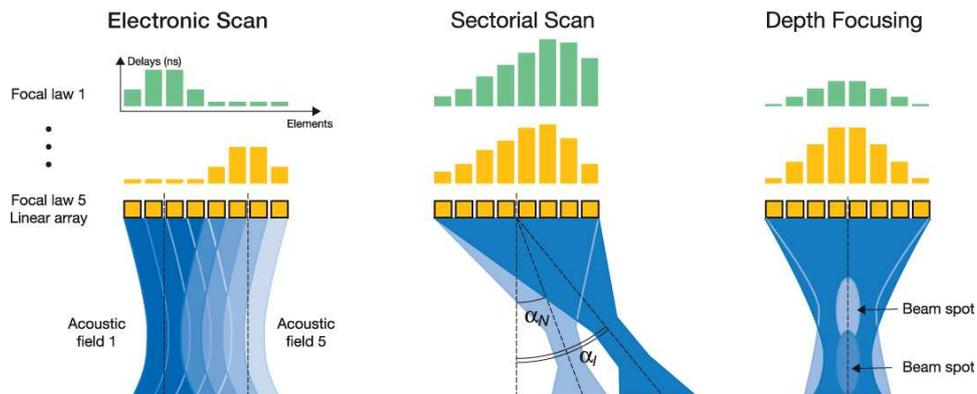
Figure 2: Schematic showing generation of electronic (originally called "linear scans") and sectorial scans using phased arrays.
