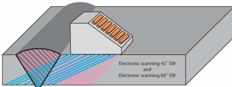
Figure 8: Schematic showing phased arrays performing ASME raster scans.
