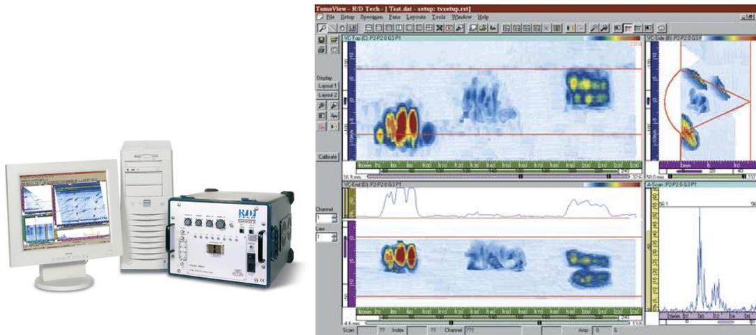
Figure 18 (left): Tomoscan III system. Figure 19 (right): “Top, side, end” view with weld overlay.
