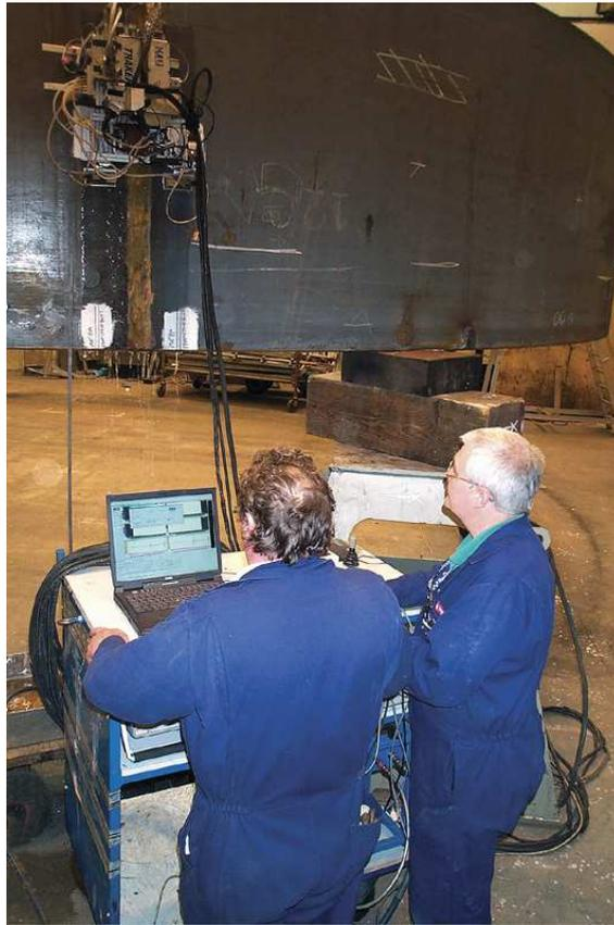
Figure 25: Magnetic wheel TRAKER inspecting vertical weld.
