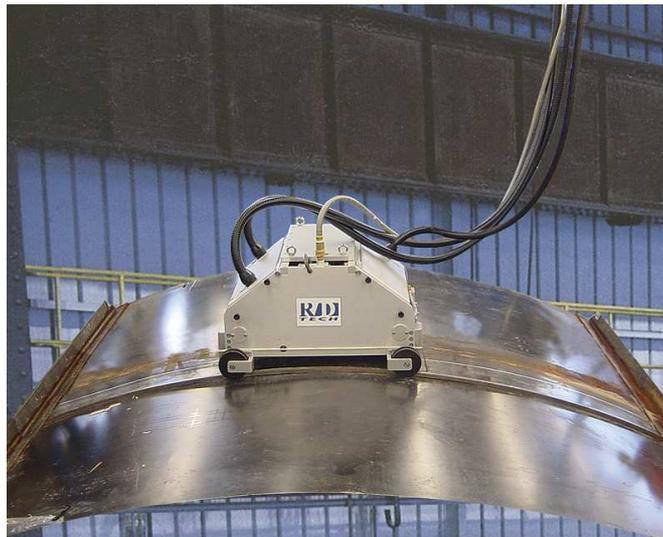
Figure 20: Typical PV-300 inspection head.
