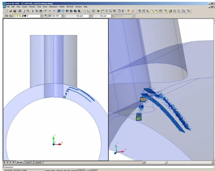
Figure 13: 3D data reconstruction of defects in nozzle (Courtesy of Zetec).
