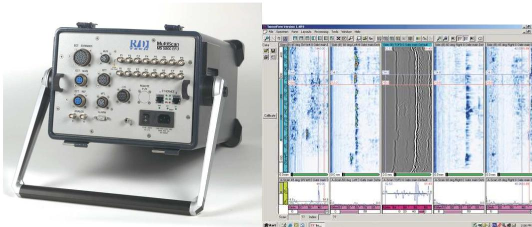
Figure 16 (left): PV-100 instrumentation. Figure 17 (right): typical PE-TOFD display.
