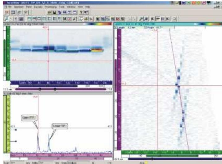
Figure 12: Typical back-diffraction scan results. Top left, C-scan; right, B-scan, bottom left, A-scan.
