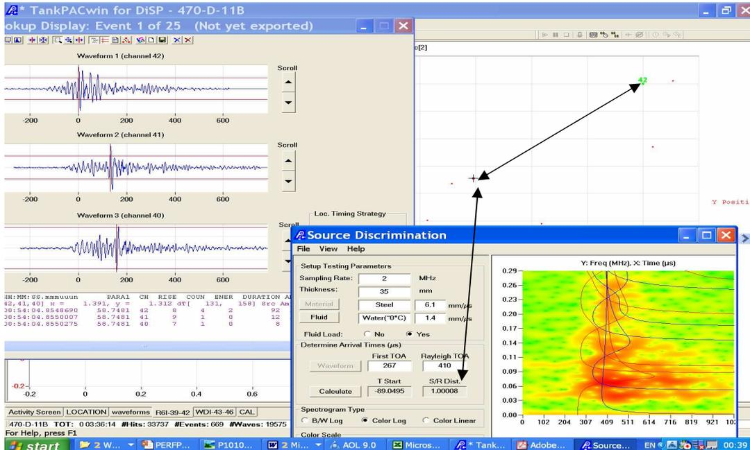
Figure 9: AE Waveforms from located source in damaged area recorded during pressurisation, source-receiver distance calculated at 1 m agrees with computed source position
