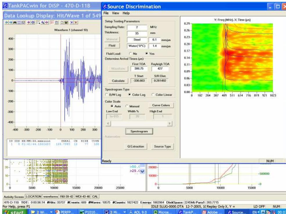
Figure 8: AE Waveform recorded during pressurisation, source-receiver distance calculated at 281 mm
