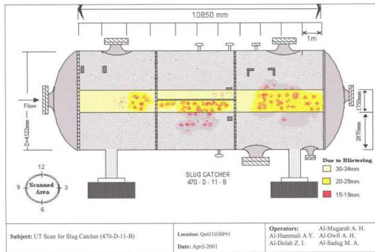
Figure 2 – Internal Ultrasonic Scanning Results
