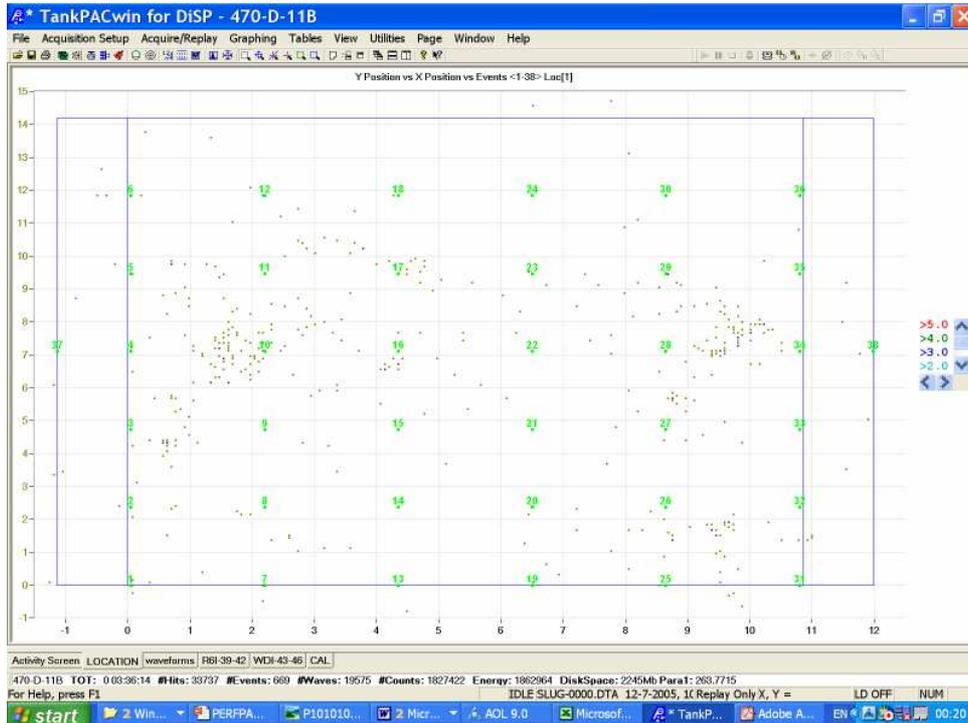
Figure 7: Planar location of vessel sources recorded during pressurisation
