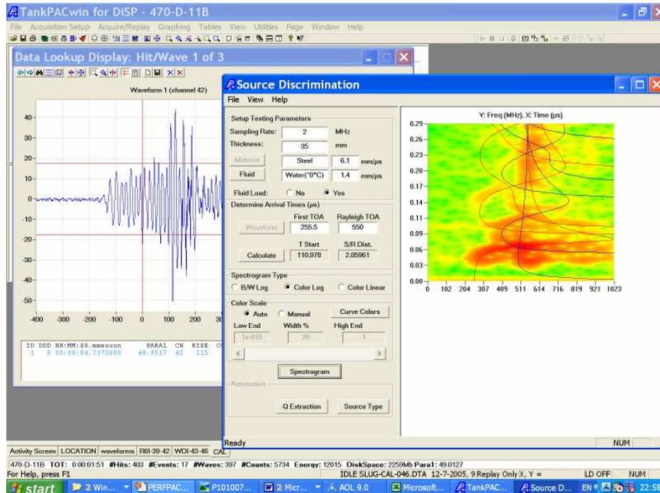
Figure 5: Hsu-Nielsen 2 mm from R6I sensor, calculated S/R distance is 2.05 metres
