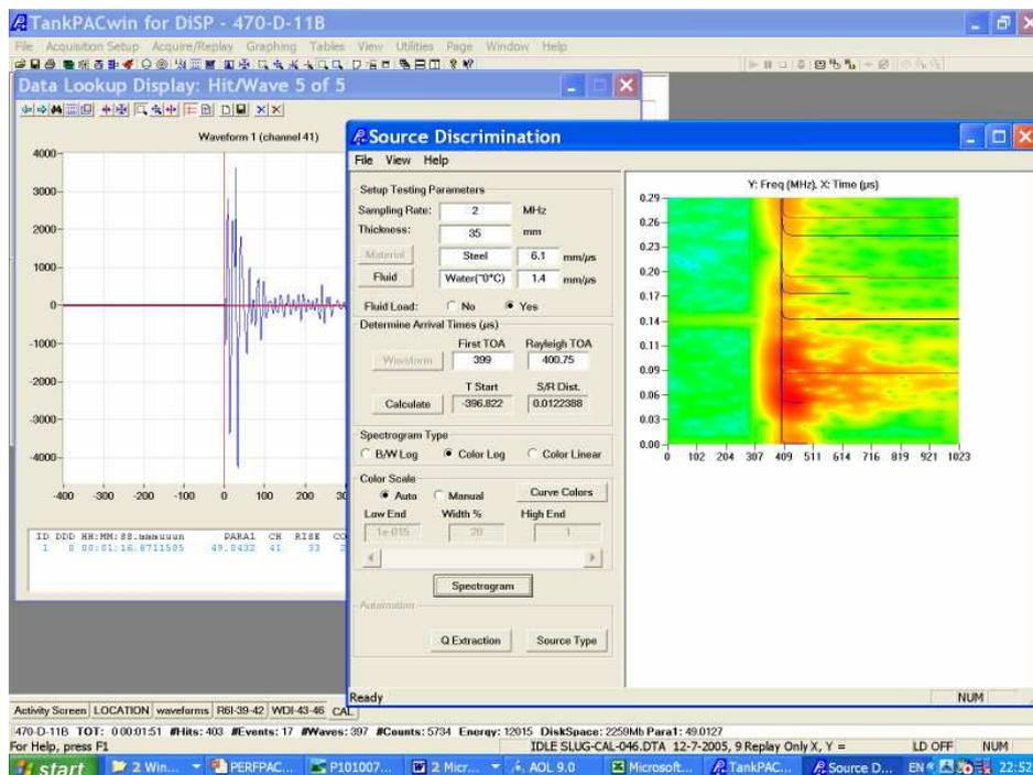
Figure 4: Hsu-Nielsen 100mm from R6I sensor, calculated S/R distance is 0.012 metres
