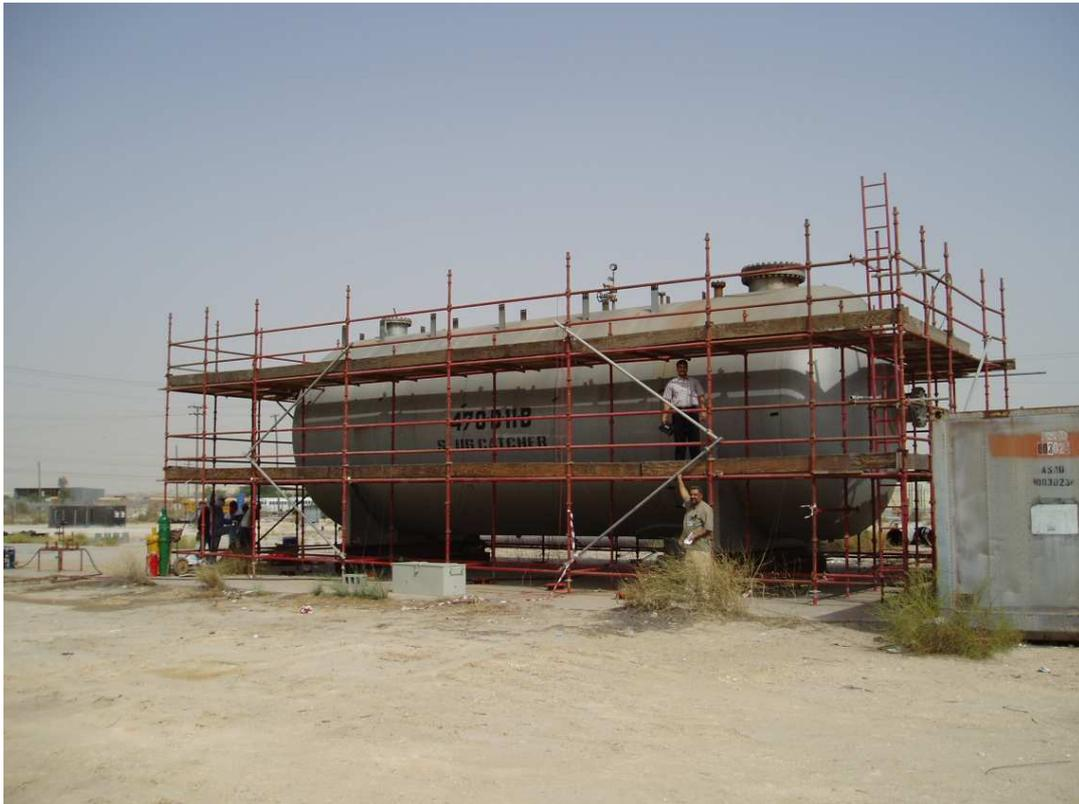
Figure 1: Slug-catcher Pressure Vessel ready for Test
