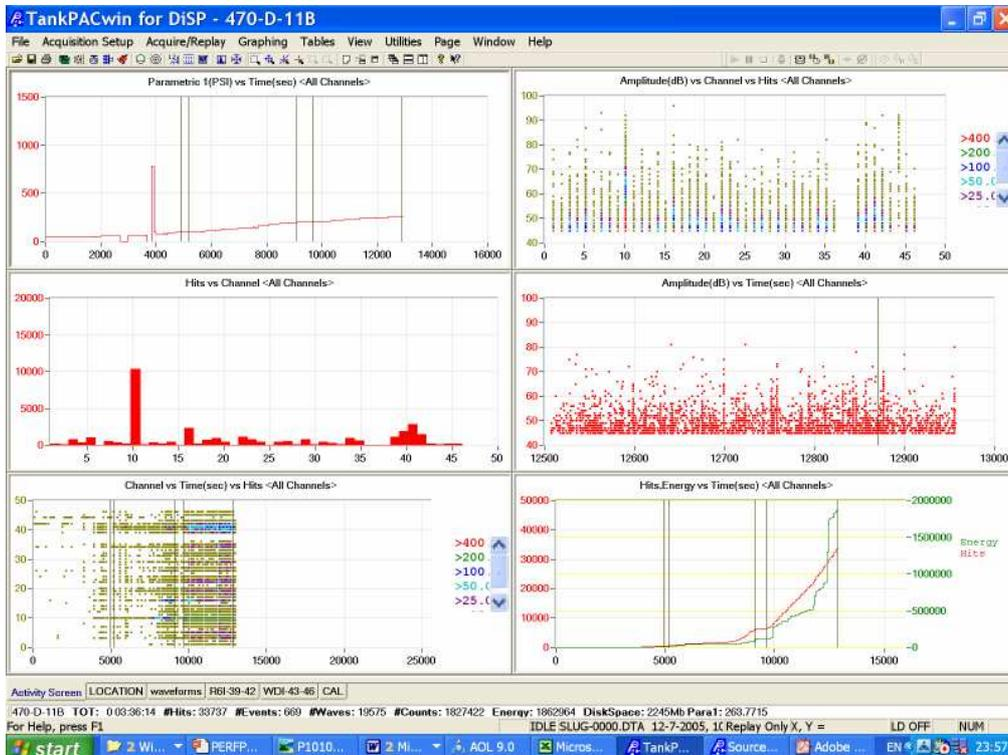
Figure 6: pressure versus time and AE feature data recorded during pressurisation
