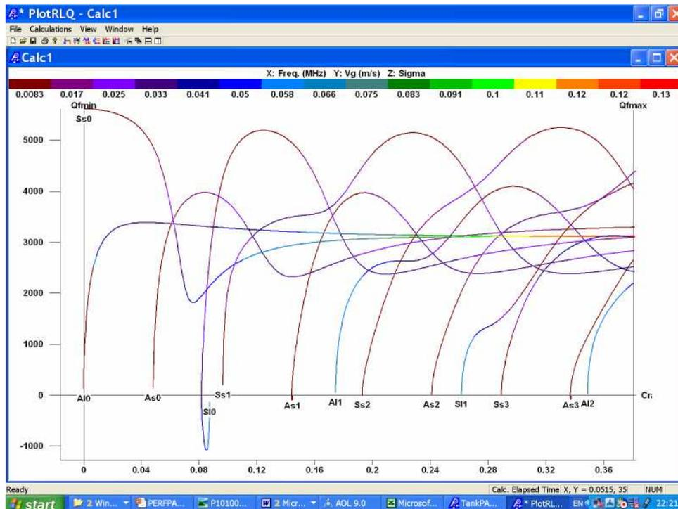
Figure 3: PLOTRLQ shows the wave modes and their attenuation, Y-axis is velocity, X-axis is MHz
