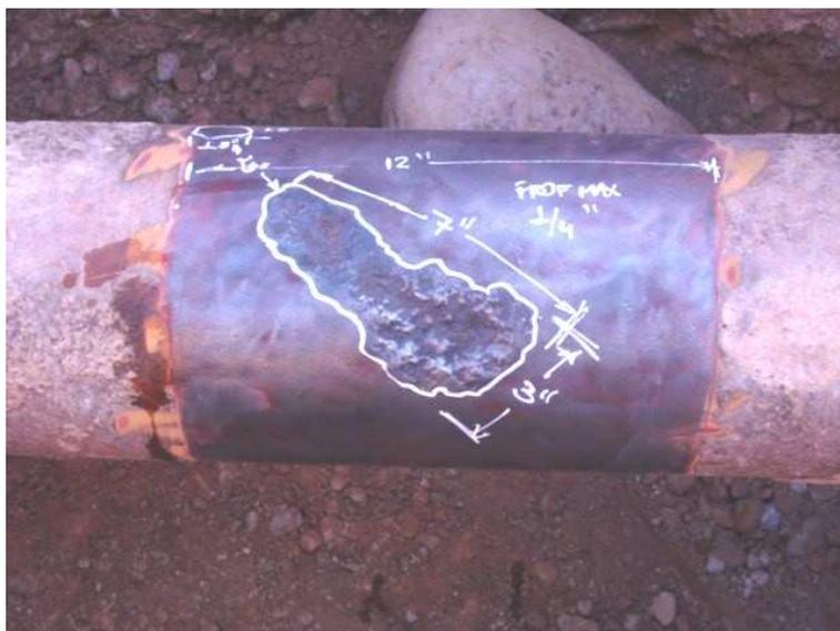
Figure 9. Corrosion patch found at exposed location about 30 meters away from the exposed location shown on Figure 7.
