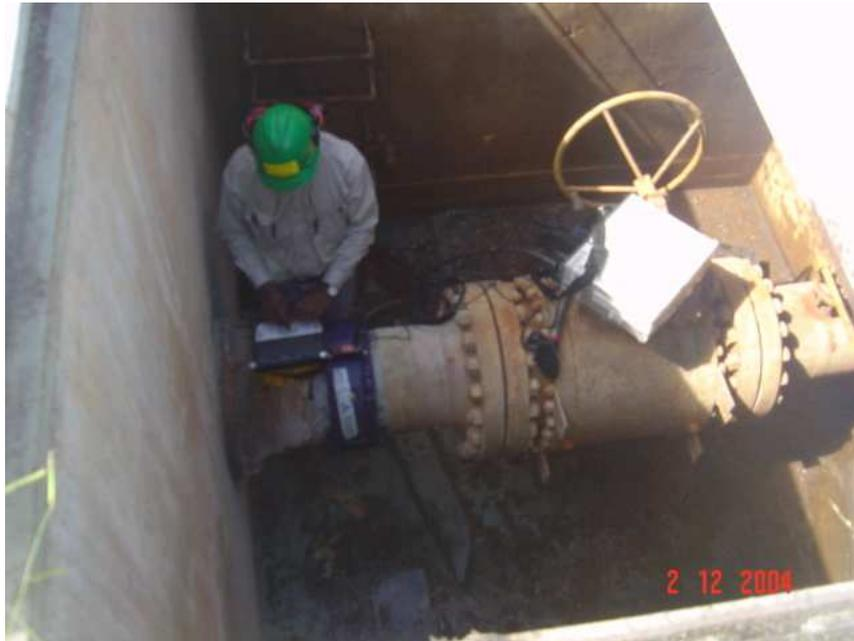
Figure 5. Wavemaker G3 in action. Test on a buried section of pipe from an accessible remote location.
