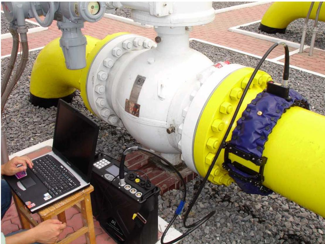
Figure 4. Wavemaker G3 kit used in site-test.
