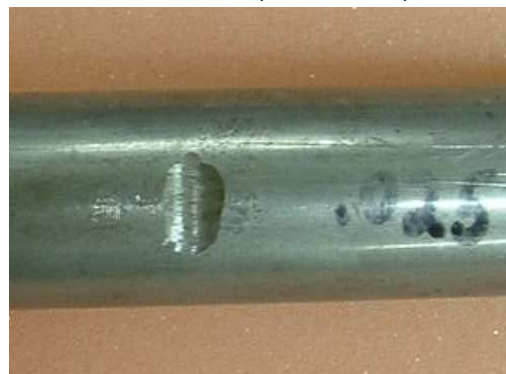
Figure 5: Pictures of the artificial defects used in the evaluation of MsS technology for heat exchanger tube inspection.
