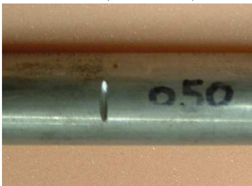
Figure 5: Pictures of the artificial defects used in the evaluation of MsS technology for heat exchanger tube inspection.
