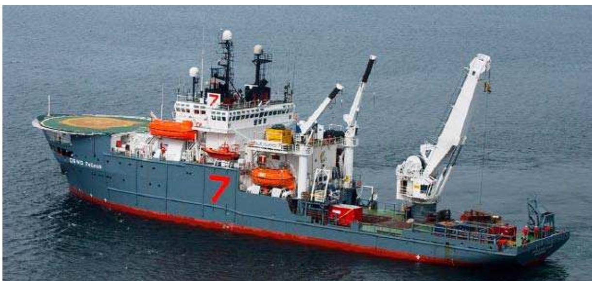
**Figure 10: The diver supply vessel (DSV) Pelican**
