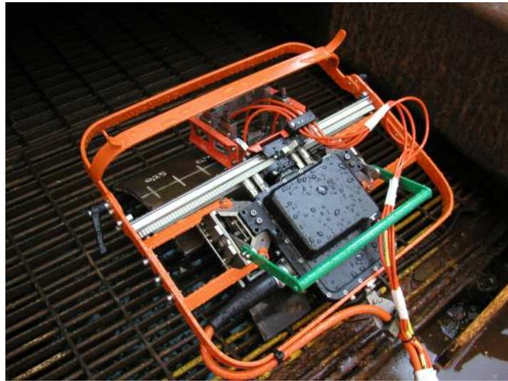
**Figure 9: Scanner AUS-4 configured for diver operation**
