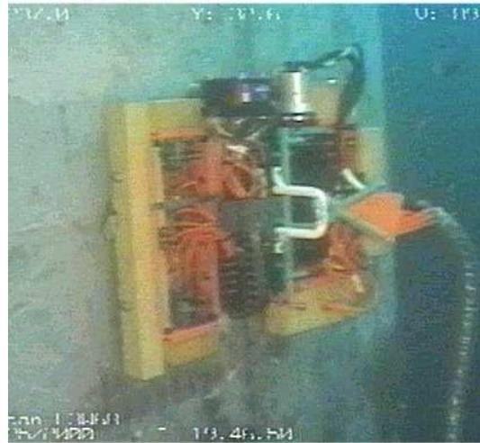
**Figure 7: Scanner AUS-4 at work subsea**
