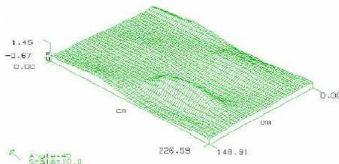
**Figure 8: Graph of dents found by calliper inspection.**
