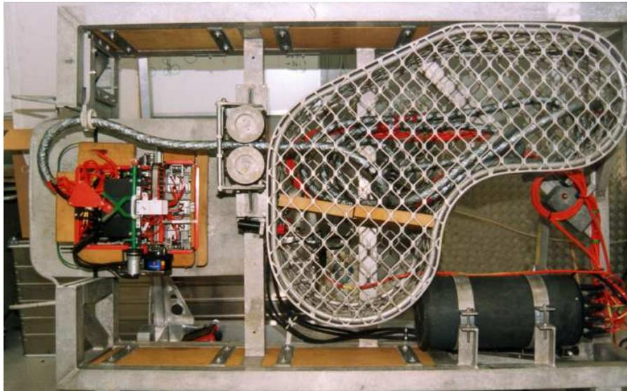
**Figure 1: Tool skid with the complete inspection system. The scanner is placed on a platform where a calibration block is integrated. The cable handling system is operated by hydraulic power supplied by the ROV. The P-scan system 4 is placed in an electronic's pressure bottle. One cable is connected to the ROV's umbilical. All communication is through this cable.**
