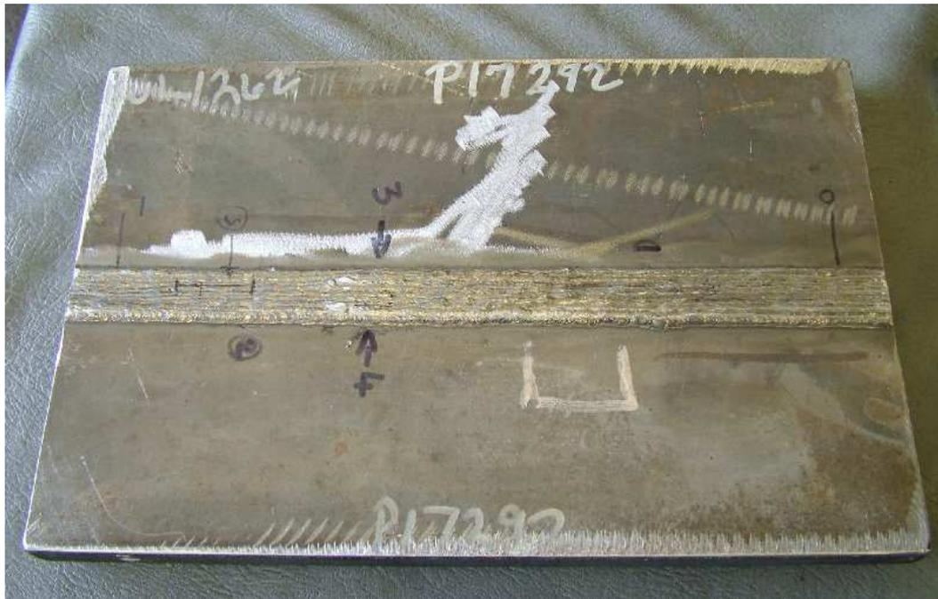
**Figure 5: Test sample for ACFM experiments**
