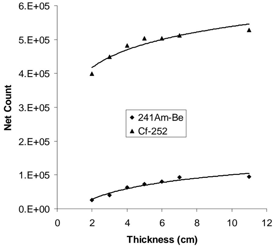
Fig. 2 : Counts for 5 minutes of back diffused neutrons vs paraffin scale thicknesses for <sup>241</sup>Am-Be and <sup>252</sup>Cf sources; the pipe wall thickness was 4 mm.
