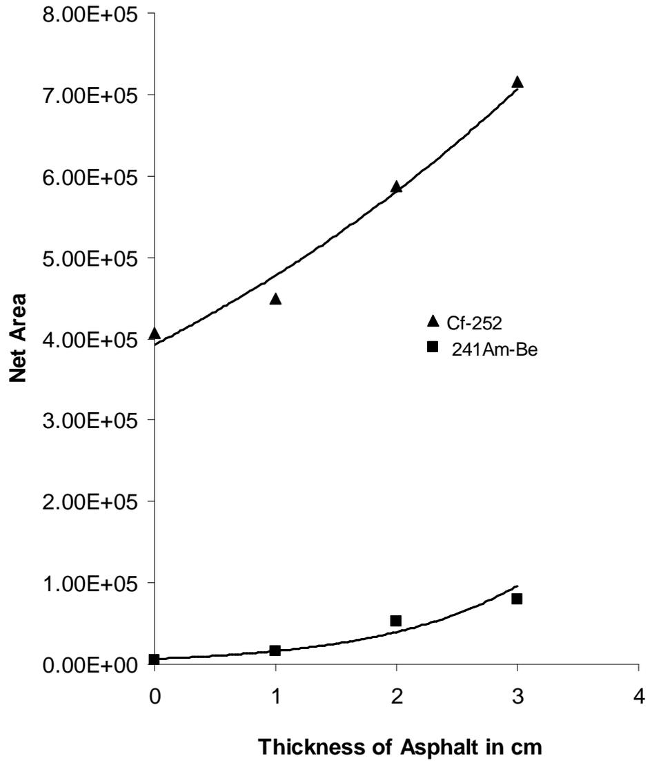
Fig. 3 : Counts for 5 minutes of back diffused neutron vs asphalt scale thickness using  $^{241}\text{Am-Be}$  source; the pipe wall thickness was 4 mm.
