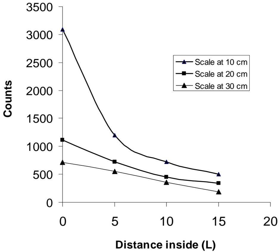
Fig. 8 : Counts in  $\text{BF}_3$  Counter at different distances L inside boron shield and different paraffin scale distances D of 10, 20 and 30 cm from the detection system.
