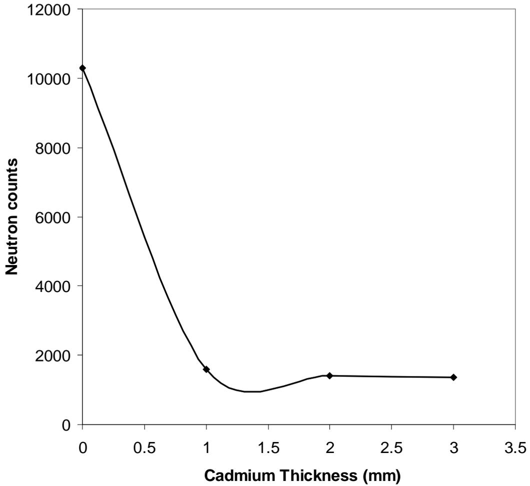
Fig. 4 : Neutron Counts for 2 min from  $^{252}\text{Cf}$  source for different thickness of Cadmium around the  $\text{BF}_3$  detector
