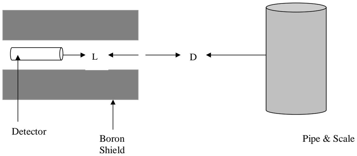
Fig. 7: Geometry for collimation measurements
