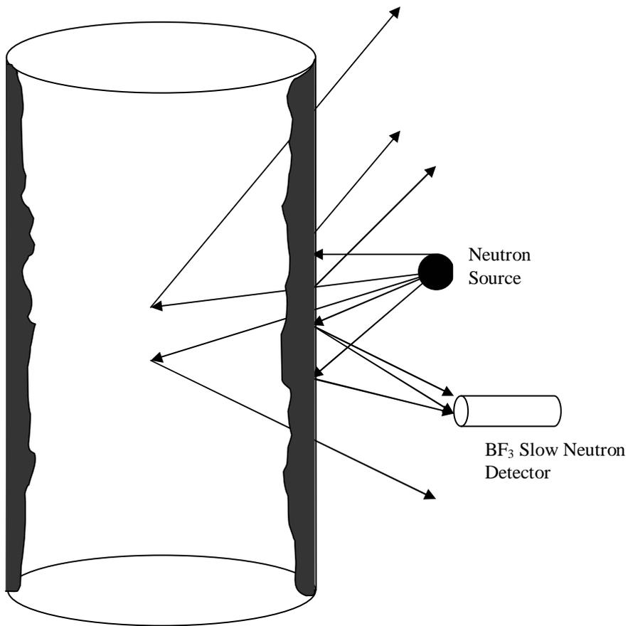
Fig.1 Neutron back scattering and back diffusion
