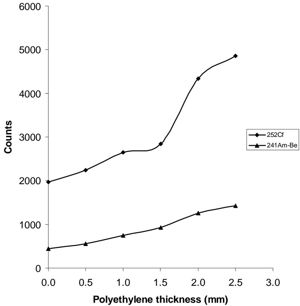
Fig. 9: Neutron counts for 10 min in  $\text{BF}_3$  counter held horizontally and surrounded by 2.5 cm boron at 2 cm away from polyethylene scale inside iron pipe, using  $^{252}\text{Cf}$  and  $^{241}\text{Am-Be}$  sources.
