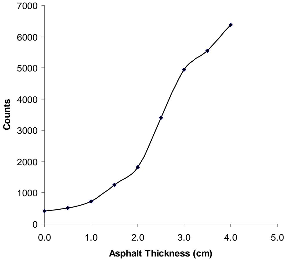
Fig. 6 :Counts for 2 min in vertically positioned  $\text{BF}_3$  detector surrounded by 2.5 cm thickness of boron with 1 cm opening at different asphalt scale thicknesses, using  $^{252}\text{Cf}$  source.
