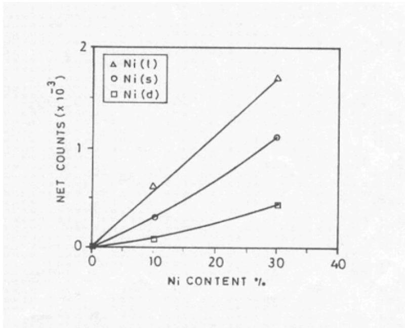
Fig. 3 Net count for 6 h of 8.999 MeV full, single escape and double escape capture gamma rays versus Ni ratio in Cu – Ni alloy.
