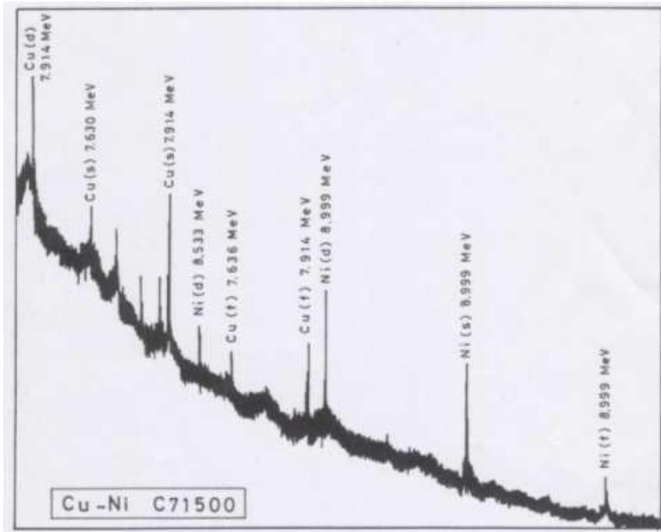
Fig. 2 Spectrum of capture gamma rays emitted from Cu- Ni alloy type C71500
