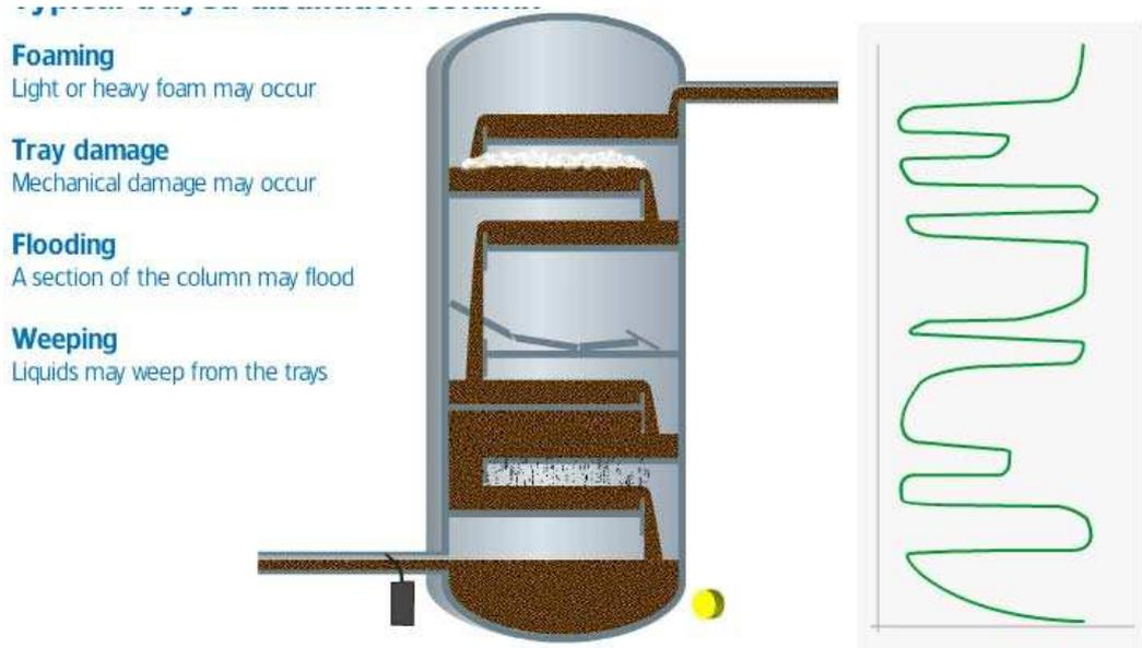
The same technique can be used for packed bed columns to establish the position of beds, and also identify any mal-distribution through the beds. By selecting a series of comparable scan lines through the bed, we can measure the mean density of material across each region and establish if mal-distribution is occurring, as shown in this example below.
