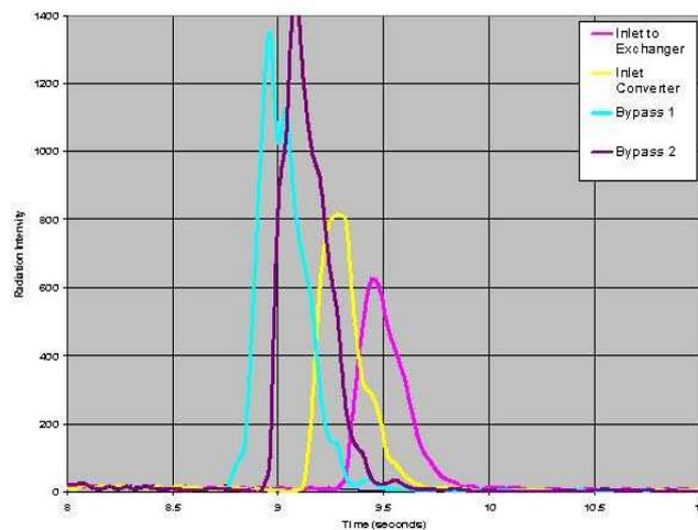
No internal bypassing was observed at the detectors on the reactor exit line, but both detectors observed leakage through the bypass valve, as shown.
