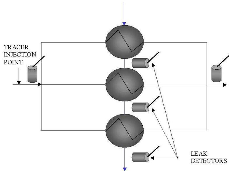
This is a very useful tool for shutdown planning purposes, so that the repairs can immediately be focussed on the exchanger that is leaking, rather than wasting valuable time and money testing each exchanger in turn during the shutdown.
