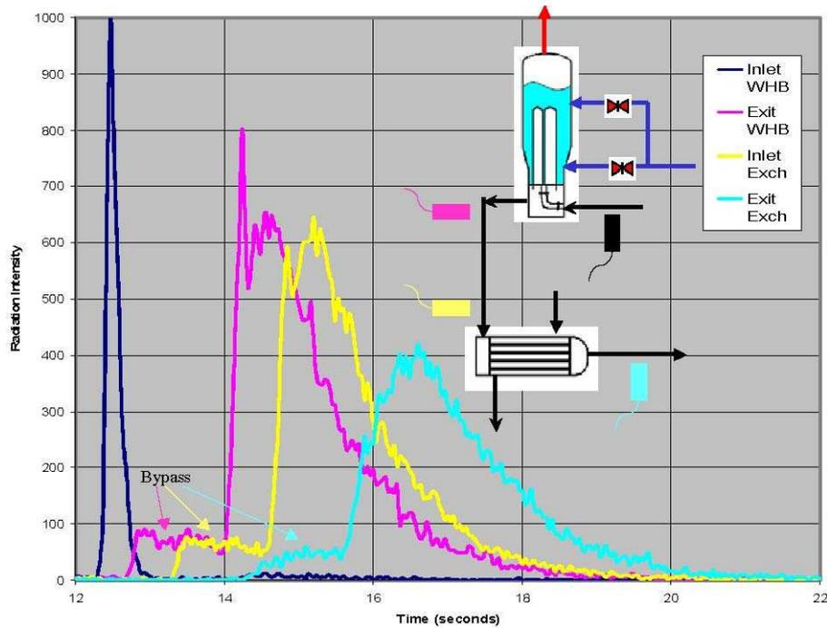
As can be seen from the graph, initial bypass peaks were observed at each detector, prior to the main pulse of tracer being observed. This conclusively proved that internal bypassing was occurring, and a replacement bellows inlet device was ordered to be installed in the forthcoming shut down.
