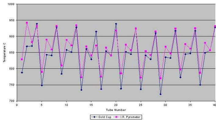
As Infrared pyrometers tend to give tube wall temperature readings that are higher than the actual temperature (typically 30 to 50 degrees Celsius), the gold cup technique enables operators to confidently increase process rates and run at higher temperatures if required, in the knowledge that tube life is not affected. The gold cup service can also be used to accurately calibrate plant IR pyrometers on site.
