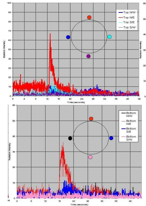
These graphs clearly show a greater response from the detectors on the North/East (N/E) side of the vessel at both the top and bottom of the bed, indicating gross mal-distribution down this side of the vessel.
