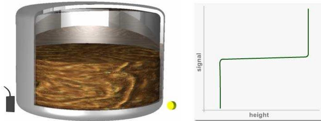
By suspending a gamma ray emitting radioactive source on one side of a vessel, and a radiation detector on the other, we can measure the amount of gamma-ray absorption at set intervals down the length of the vessel. This is effectively the mean density of material between the source and detector at each point, and hence levels can be easily and quickly identified.
