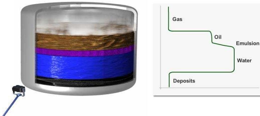
In addition to level measurements, the Neutron Backscatter technique can be used to accurately measure interfaces such as oil/water or oil/sludge, because of the differing hydrogen content between the two phases. It can also be used to measure the quality of any interface, i.e. the extent of any foam or emulsion bands. The technique is typically used on:
