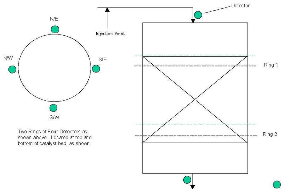
Two Rings of Four Detectors as shown above. Located at top and bottom of catalyst bed, as shown.
