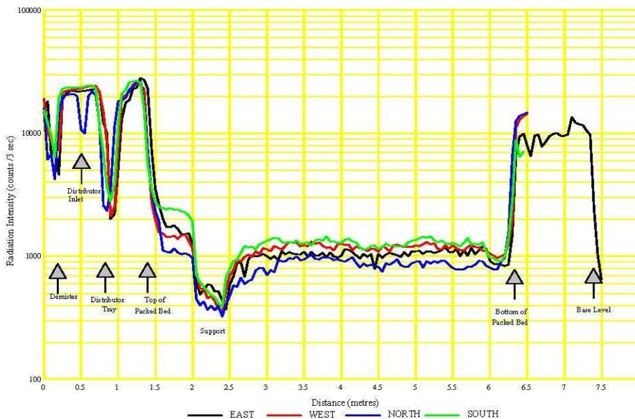
The second set of scans show the mean density of liquid through the bed to be much more uniform, and confirm that the cause of the mal-distribution was identified and repaired.
