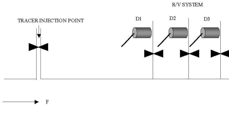
If it is suspected that valves are passing, on a relief valve system for example, a suitable radioisotope tracer can be injected upstream of the valves, and radiation detectors placed downstream of each valve under investigation as shown below. If any of the valves are leaking, the radiotracer will follow the leak and be detected by the relevant detector.
