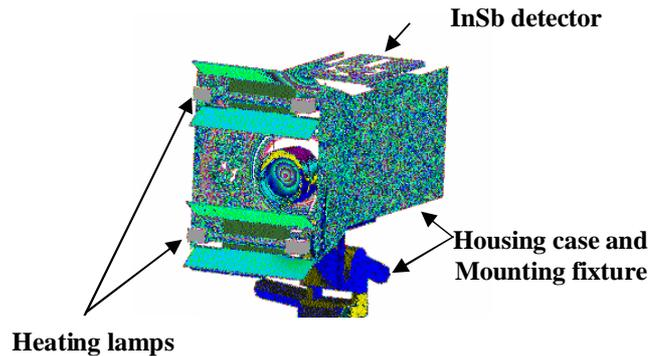
**Figure 5, The detection head used for pinhole detection**
