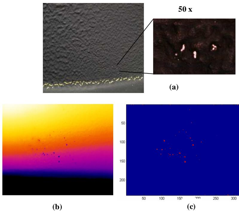
**Figure 1. Visual, thermal and post-processed images of an under coated sample container: (a) Visual image for thin spots, and under 50-x magnification. (b) Thermal image of the field view in a, and (c) Processed image**
