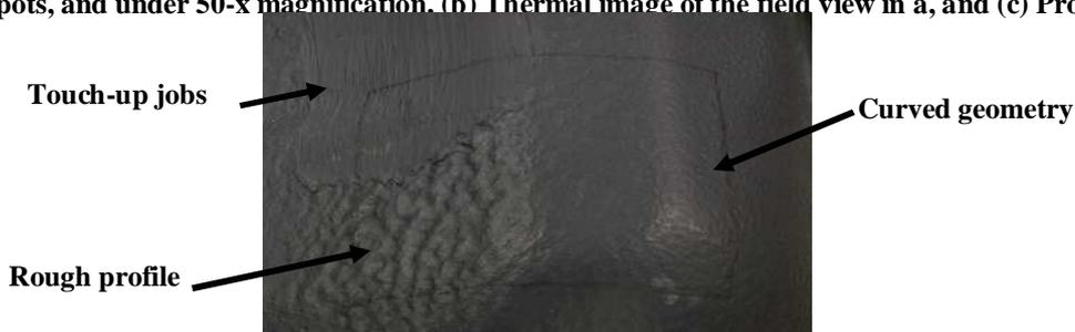
**Figure 2. A color photograph showing surface profile of coated container**
