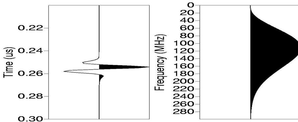
**Figure 1: The source pulse (left) and its frequency content (right). The source pulse has a peak frequency of 110 MHz.**
