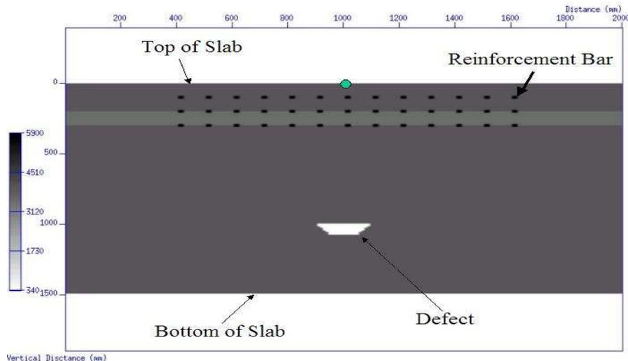
**Figure 5: An acoustic velocity model of the Slab used to numerically generate acoustic waves similar to those used in the IE test. The point in the middle is the location of the acquisition of IE in Figure 6.**
