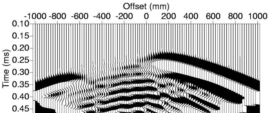
**Figure 8: The synthetic section corresponding to an excitation of a source pulse with peak frequency of 13.5 KHz in the model shown in Figure 7.**
