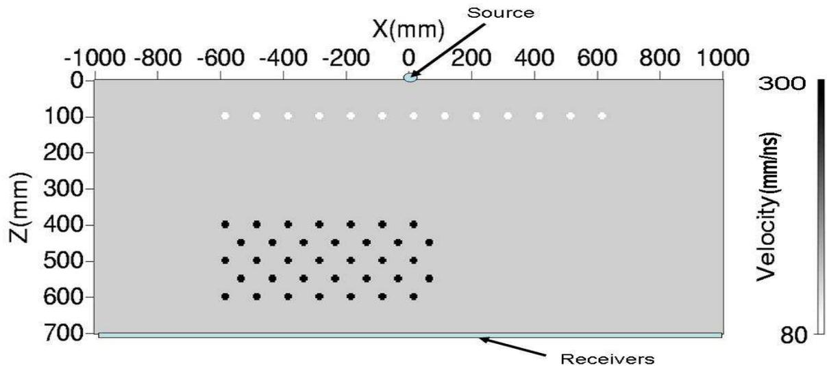
**Figure 11: A model emulating a concrete slab with reinforcement towards the top and air-filled voids towards the bottom. The source is located on the middle of the top surface and the receivers are located along the whole model on the bottom. The velocities here of the materials are for electromagnetic waves.**
