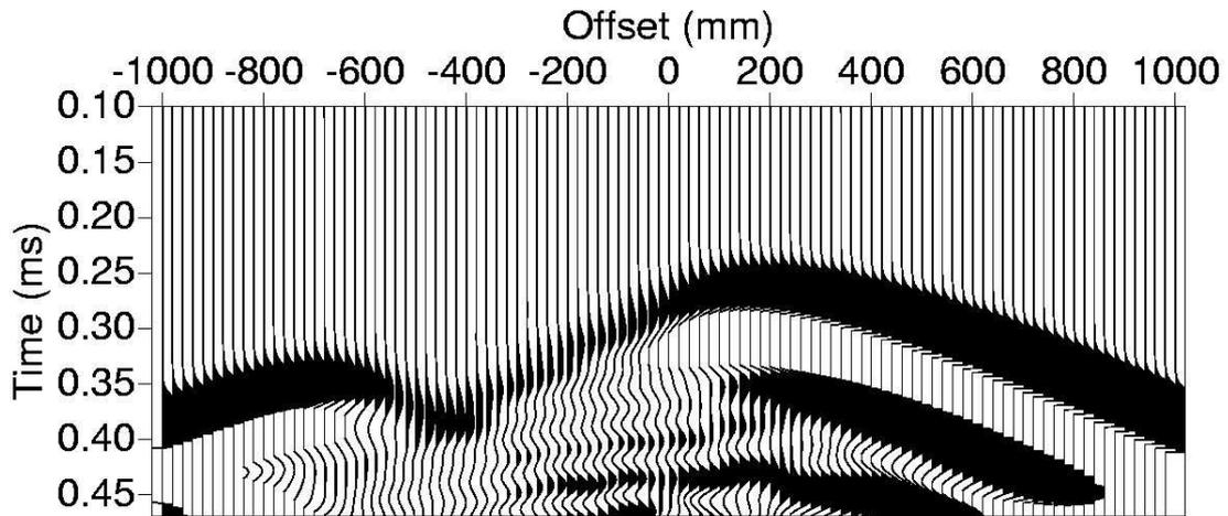
**Figure 9: The synthetic section corresponding to an excitation of a source pulse with peak frequency of 9.3 KHz for in model shown in Figure 7.**
