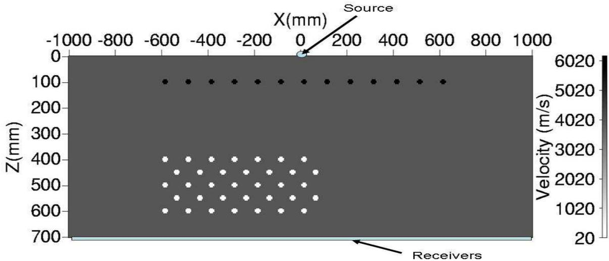
**Figure 7: A model emulating a concrete slab with reinforcement towards the top and air-filled voids towards the bottom. The source is located on the middle of the top surface and the receivers are located along the whole model on the bottom. The model is given in terms of seismic velocities.**
