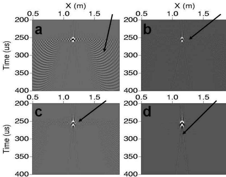
Figure 3: The recovered image using zero-offset migration applied to (a) the synthetic data of a diffractor in Figure 2, (b) a similar synthetic data with twice the sampling points (sampling interval of 1 cm) in the lateral direction, (c) a similar synthetic data but with the same sampling interval as in (b) but twice the lateral range, and (d) a similar synthetic data with the larger range as in (c), but with double the sampling points (sampling interval of 0.5 cm).
