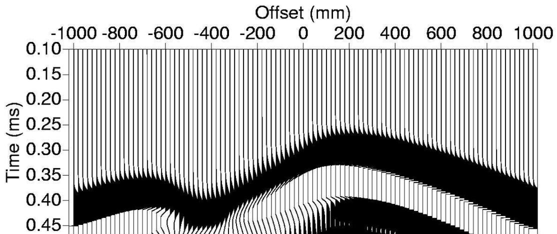
**Figure 10: The synthetic section corresponding to an excitation of a source pulse with peak frequency of 6.5 KHz in the model shown in Figure 7.**
