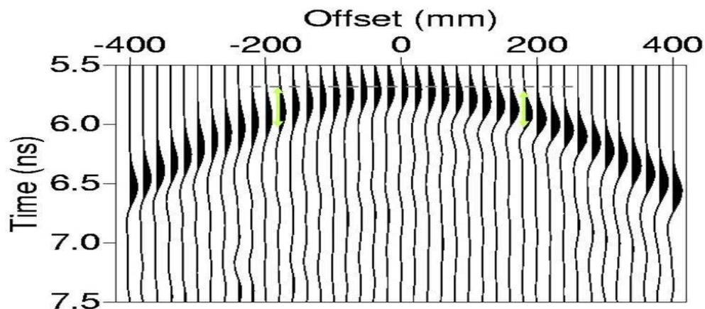
**Figure 12: The synthetic section corresponding to an excitation of a source pulse with peak frequency of 1.4 GHz in the model shown in Figure 11. The arrows clarify the time length of the wave and its time location.**
