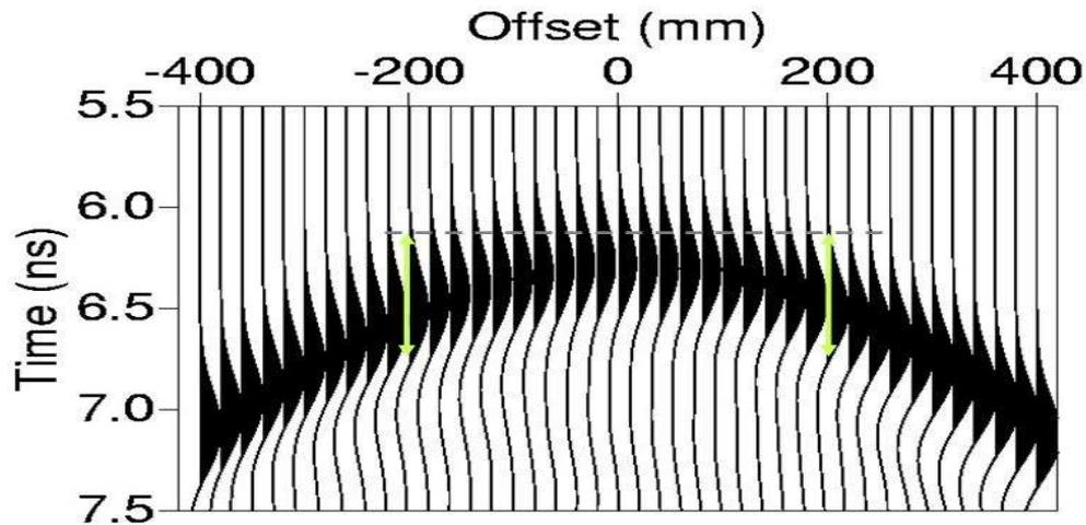
**Figure 13: The synthetic section corresponding to an excitation of a source pulse with peak frequency of 0.8 GHz in the model shown in Figure 11. The arrows clarify the time length of the wave and its time location.**
