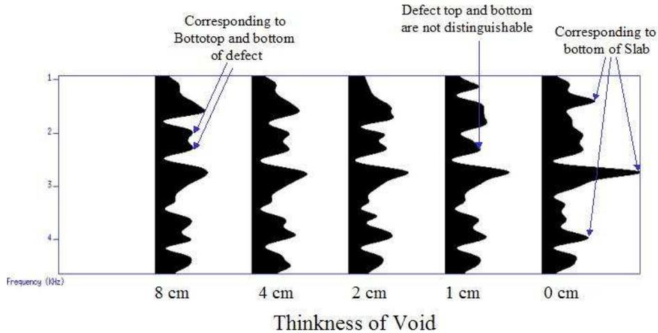
**Figure 6: The spectrum response of the measured acoustic trace for various thickness of the void.**
