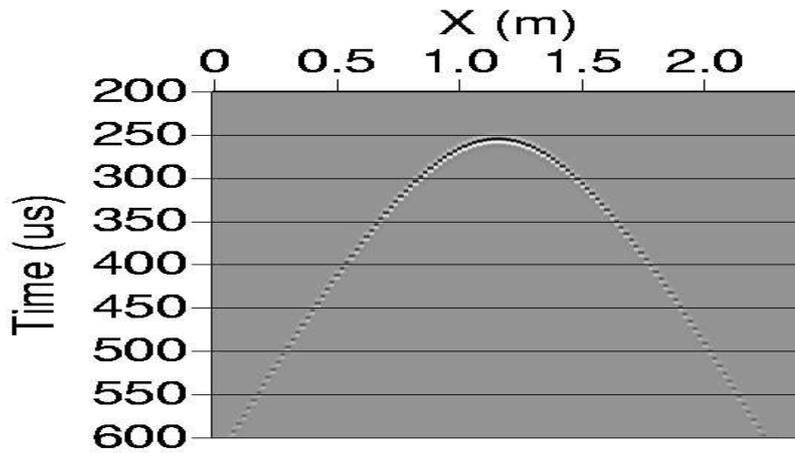
Figure 2: A section through the diffractor with a sampling of 2 cm and an offset between the source and receiver of 20 cm.
