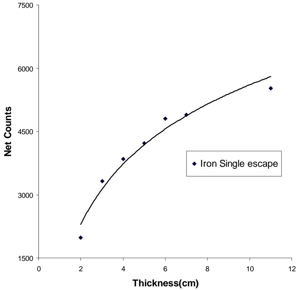
Fig. 6 :Counts for 1 hr of iron 7.63 MeV gamma ray first escape of 4 mm wall thickness pipe at differnt paraffin thicknesses, using  $^{241}\text{Am}$ -Be source.
