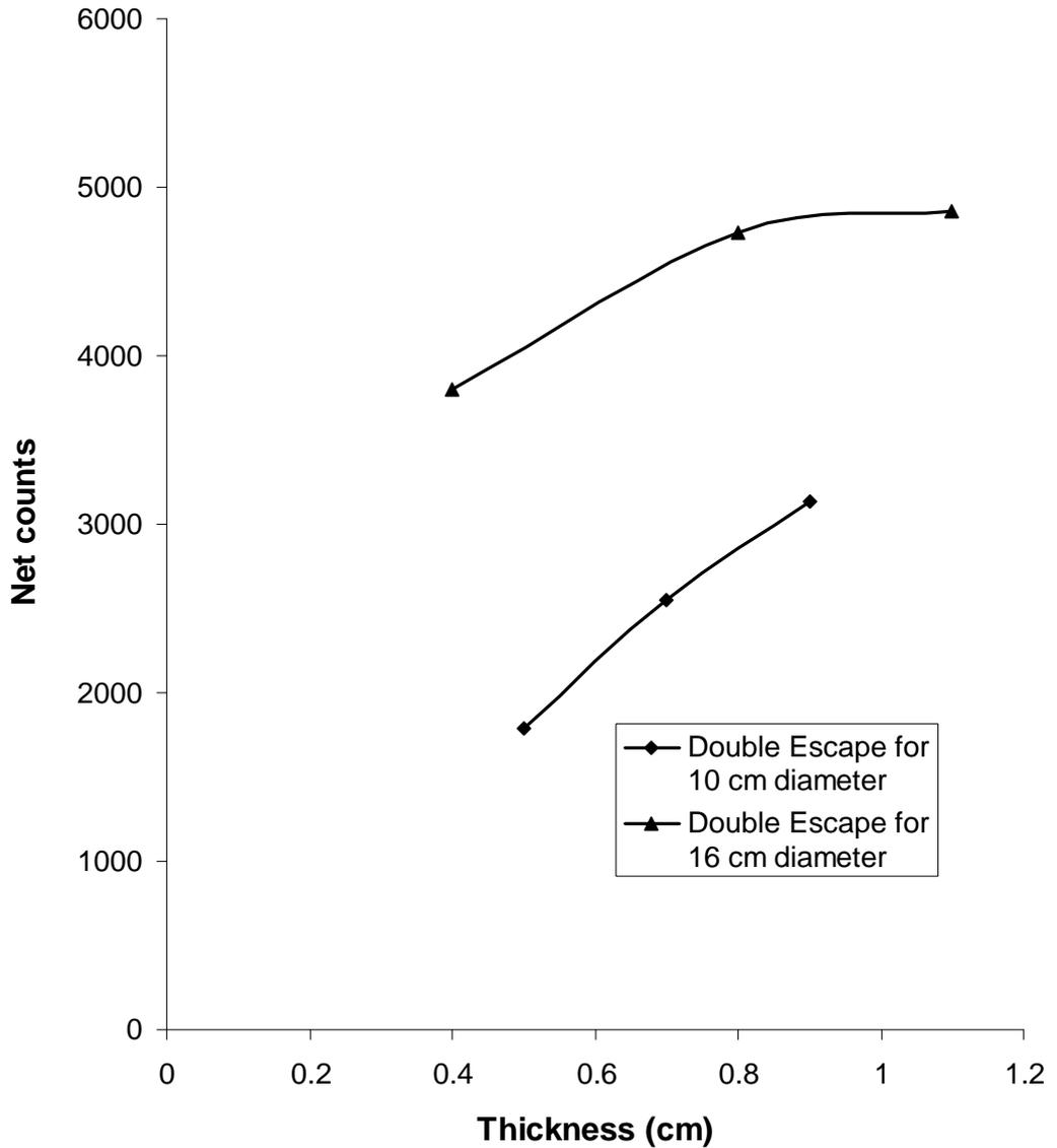
Fig. 3 : Counts for 1 h of double escape Iron 7.63 MeV gamma ray peak at wall thicknesses of 10 cm and 16 cm diameter pipes using  $^{241}\text{Am}$ -Be source. Pipe was surrounded on 3 side by water.
