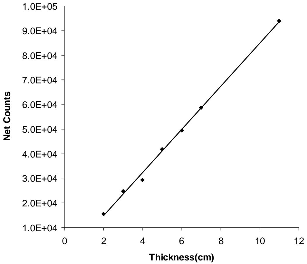
Fig. 5 :Counts for 1h of hydrogen 2.22 MeV gamma ray at different paraffin scale thicknesses, using  $^{241}\text{Am}$ -Be source.
