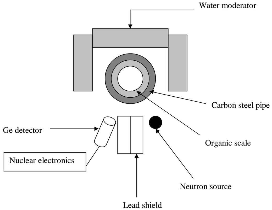
Fig. 1. Experimental set-up for neutron capture gamma ray experiment
