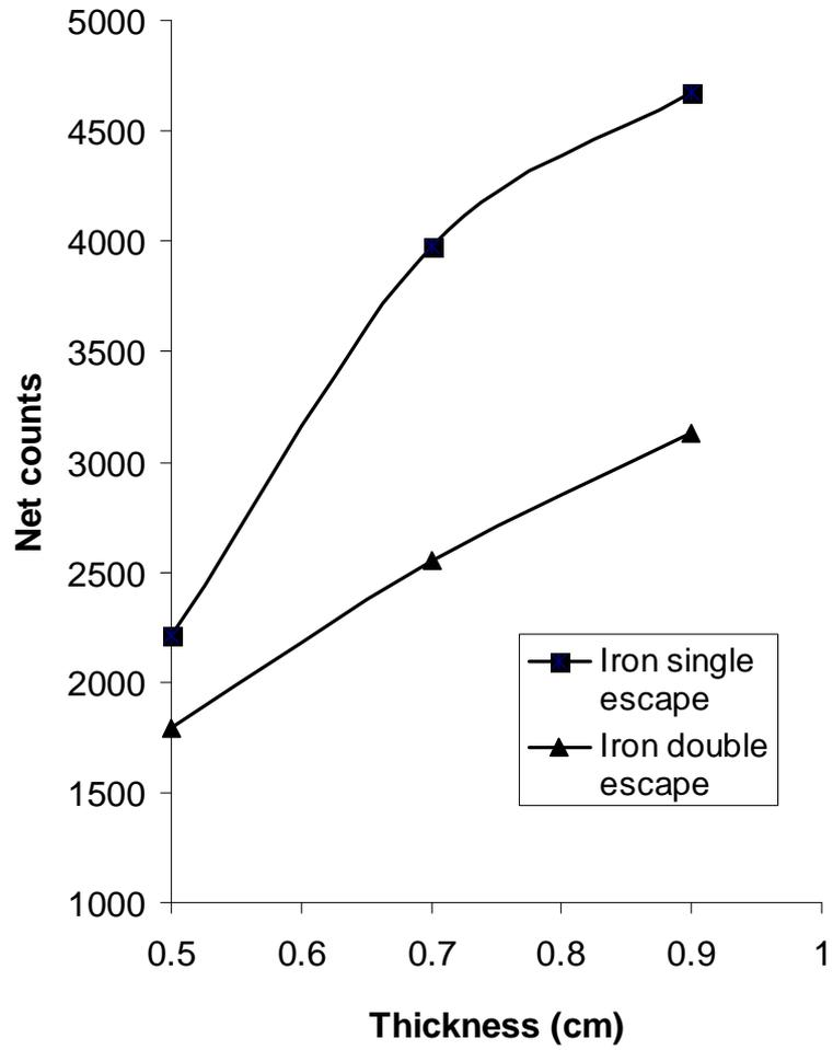
Fig. 2 : Counts for 1 hr of iron 7.6 MeV gamma ray single escape and double escape at different iron pipe thicknesses; pipe was surrounded on 3 side by water, using  $^{241}\text{Am-Be}$  source
