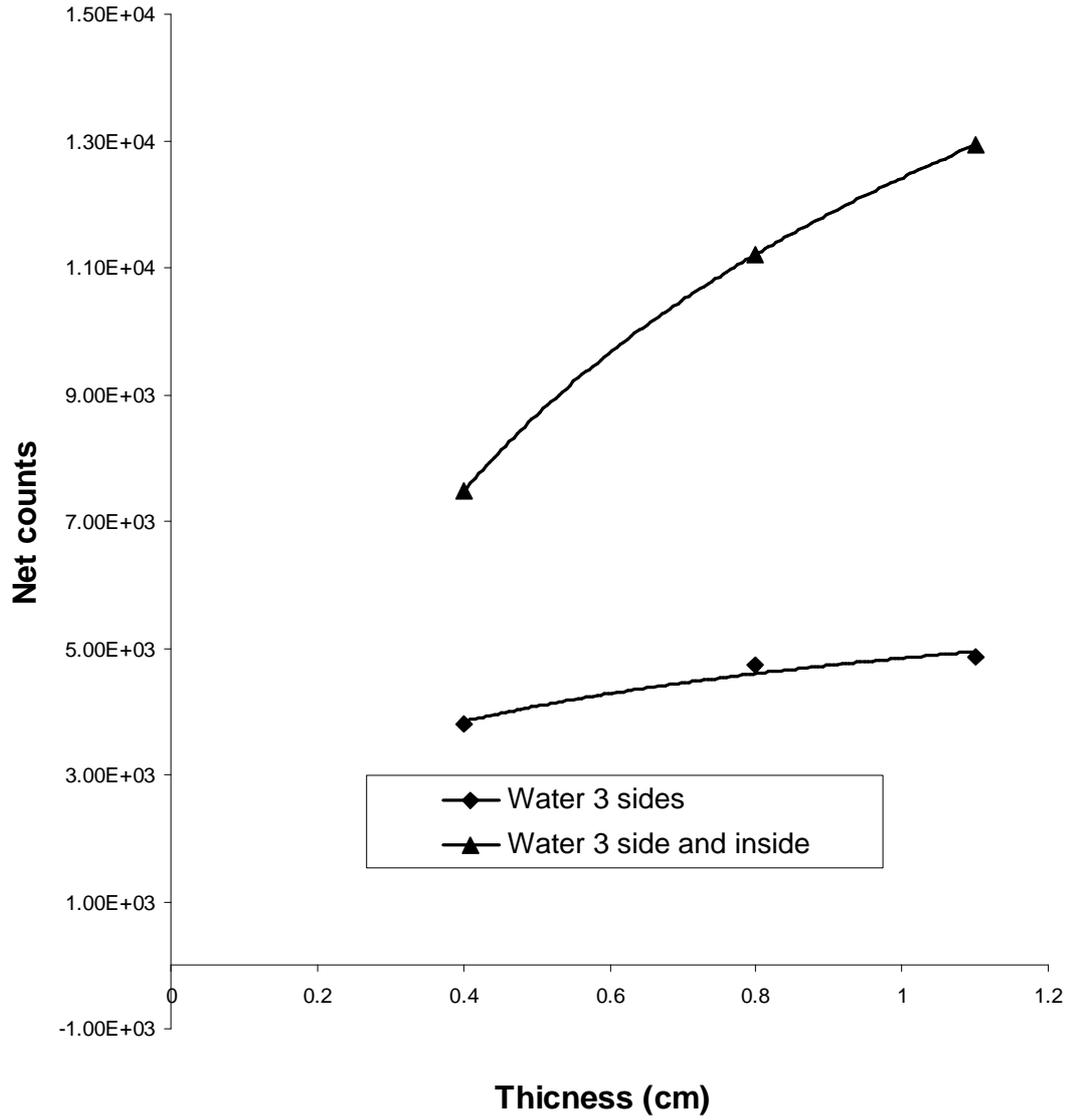
Fig. 4 : Counts of iron 7.63 MeV gamma ray double escape for 1h of 16 cm diameter pipe filled with water and for pipe filled and surrounded from 3 sides by water, using <sup>241</sup>Am-Be source.
