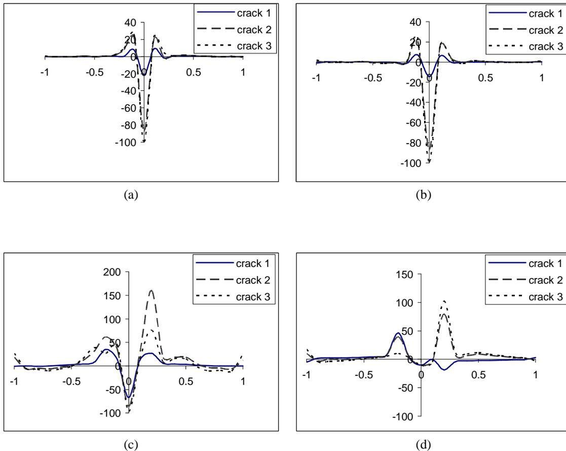
Fig. 5. Variation of normal component of  $\underline{B}$  along a path 0.4 mm on top of the connector surface with three different subsurface cracks. The operating frequencies are 100 Hz (a), 1 kHz (b), 10 kHz (c) and 50 kHz (d).
