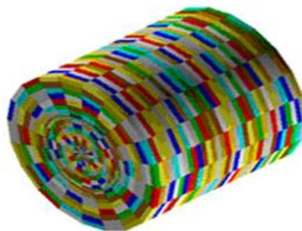
Fig. 4. Discretization of structure into 3D elements.
