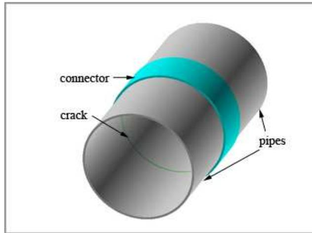
Fig. 1. Pipeline configuration with crack
