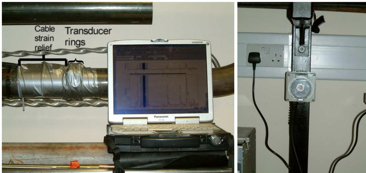
**Figure 1 Permanently installed transducer on test pipe showing low profile of design and remote connection box.**
