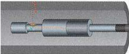
Figure 5A - Schematic of IRIS probe
