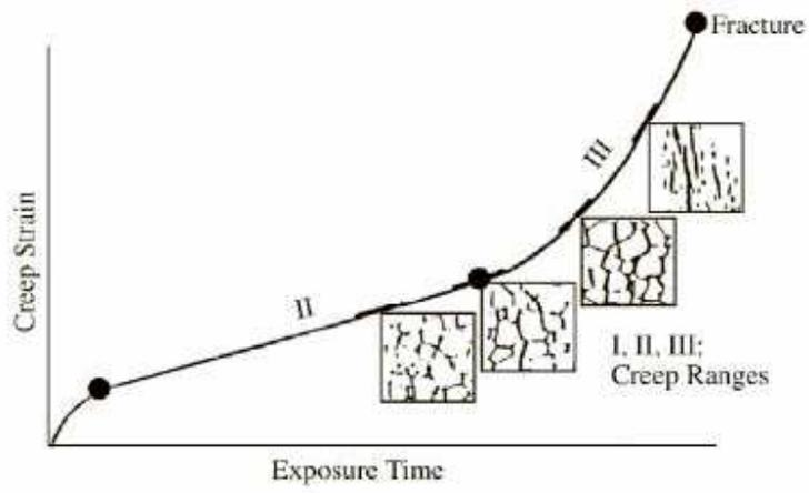
Sketch:3 Different stage of creep along with microstructure degradation stages
